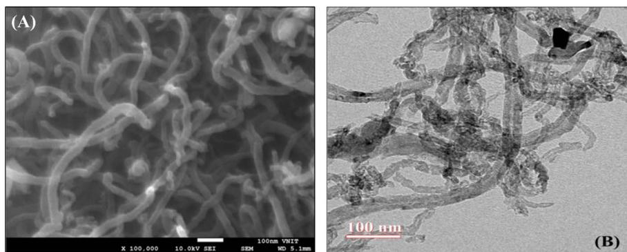
Fig. 2 (A) SEM and (B) HRTEM images of MWCNTs synthesized from waste toner powder. Reproduced from ref. 53 with permission from Taylor & Francis Group, LLC, copyright 2019.<sup>53</sup>
