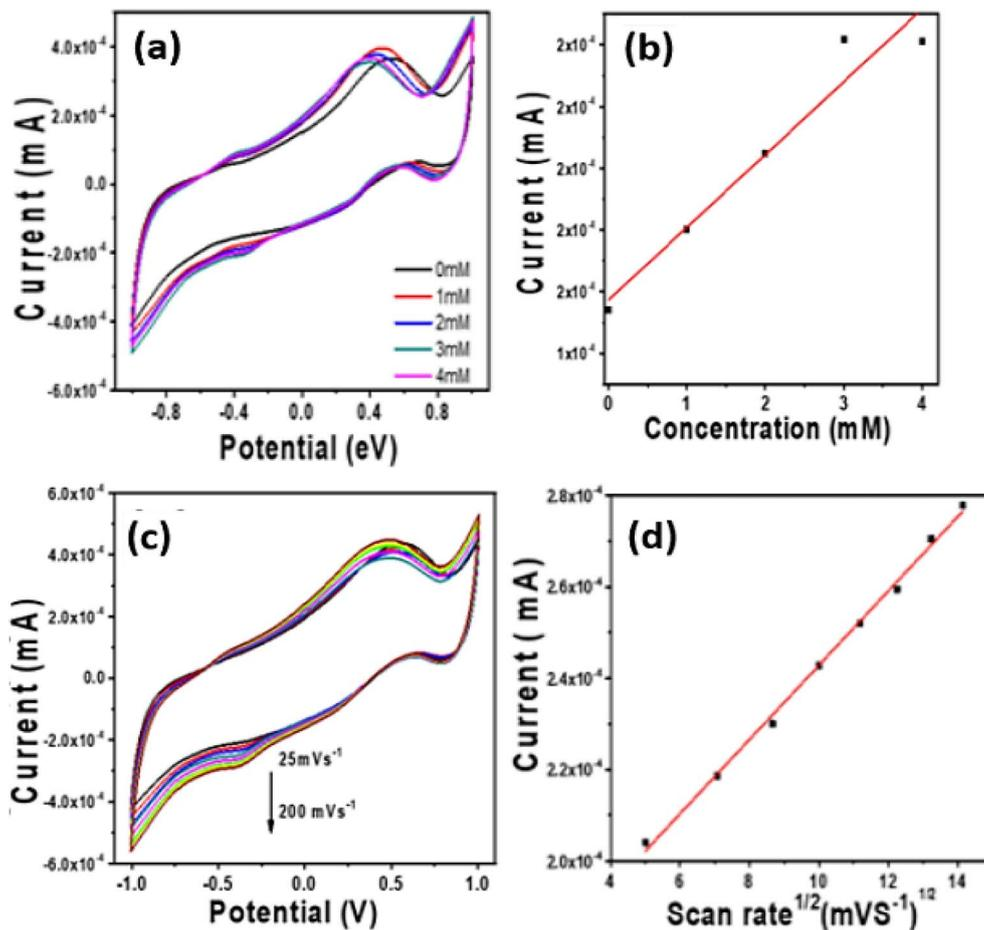
Fig. 7 (a) CVs for CoS-NR/rGO at various 4-NP concentrations (0–4 mM), (b) dependence of reduction peak currents at  $-0.35$  V on 4-NP concentrations, (c) CV curves for CoS-NR/rGO sensor at different scan rates, and (d) linear fitting of reduction peak currents at  $-0.35$  V to  $\nu^{1/2}$ .
