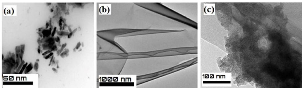
Fig. 2 TEM micrograph for (a) CoS-NR, (b) rGO, and (c) CoS-NR/rGO.
