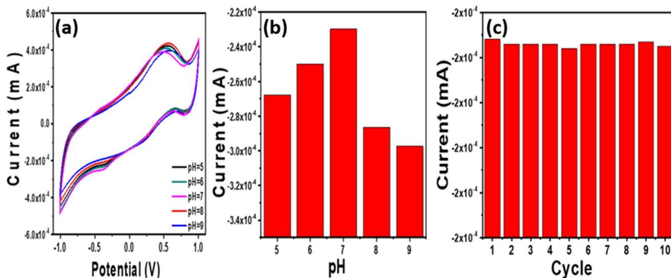
Fig. 8 (a) CVs of CoS-NR/rGO at different pH values in presence of 4 mM 4-NP, (b) dependence of reduction peak currents at  $-0.35$  V on pH, (c) effect of repeated cycling (10 cycles) of 4 mM of 4-NP at CoS-NR/rGO electrode.
