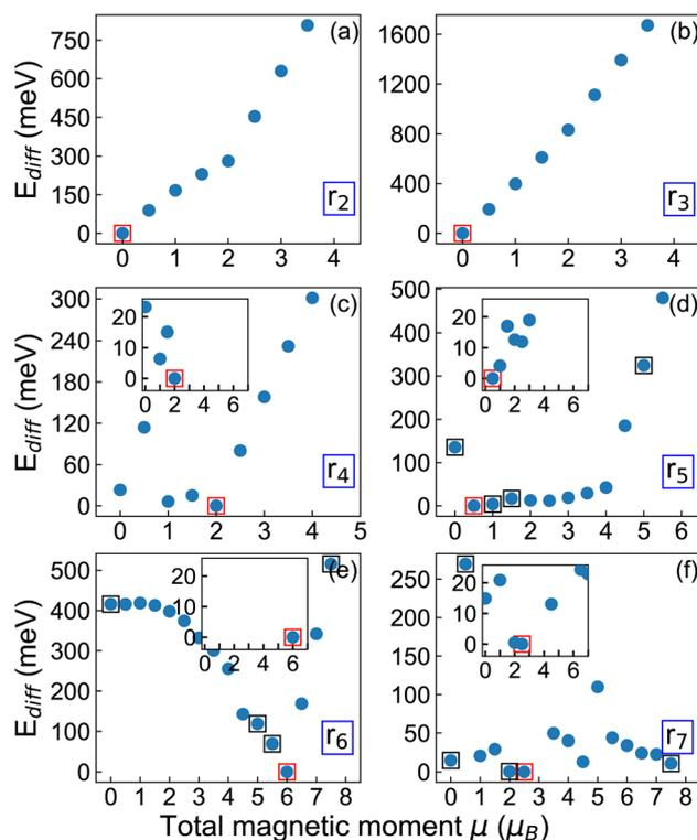
Fig. 2 (a–f) Total energy difference ( $E_{\text{diff}}$ ) relative to the magnetic ground state (red square) for various fixed total magnetic moments ( $\mu$ ) of the considered r<sub>2</sub>–r<sub>7</sub> MoS<sub>2</sub> nanoflake. Less stable configurations discussed in the text are squared in black. Insets: zoom-in to nearly degenerate magnetic orderings.
