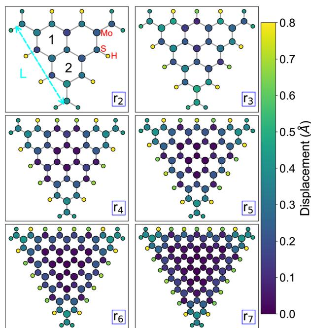
Fig. 1 Hydrogen-passivated triangular MoS<sub>2</sub> nanoflakes, with an increasing number of rings along the edge length ( $L$ ) and labeled according to them. The atoms are color-coded according to the magnitude of their displacement from the initial positions after structural optimization.
