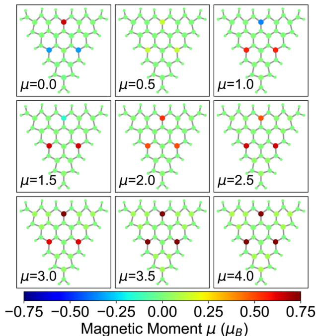
Fig. 3 Spatial distribution of the local magnetic moments in the  $r_4$  nanoflake at varying total magnetization (in  $\mu_B$ ) indicated in each panel. The color scale for the atoms represents the magnitude and orientation of the local spins.
