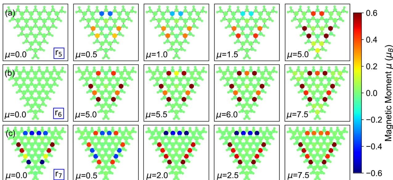
Fig. 4 Spatial distribution of the local magnetic moments in selected (a)  $r_5$ , (b)  $r_6$ , and (c)  $r_7$  magnetic configurations. The color scale for the atoms represents the magnitude and orientation of the local spins.
