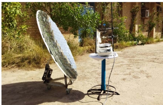
Fig. 2 CSR assembly used for the synthesis of BZI derivatives.
