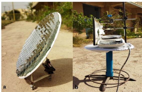
Fig. 3 Components of the CSR system: (a) reflector and (b) turret used for synthesizing BZI derivatives.
