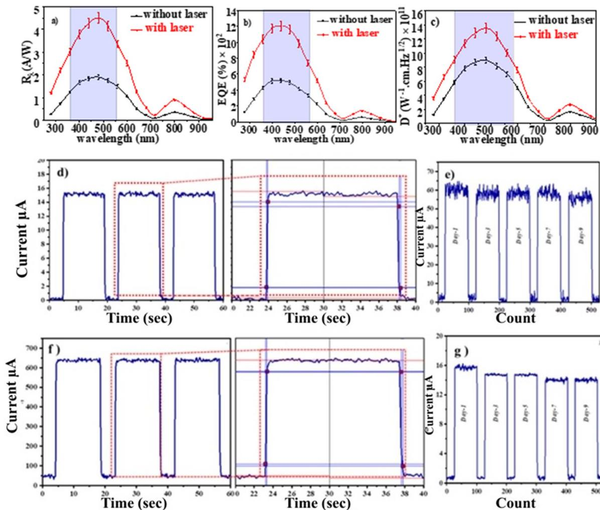
**Fig. 5** Figure-of-merits of CdS/PSi photodetectors, including (a) responsivity ( $R_s$ ), (b) external quantum efficiency (EQE), and (c) specific detectivity ( $D^*$ ). The time-dependence characteristics and stability profiles of these photodetectors at 3 V bias voltage are shown in (d) and (e) without laser, in (f) and (g) with laser of intensity of  $10 \text{ mW cm}^{-2}$ .
