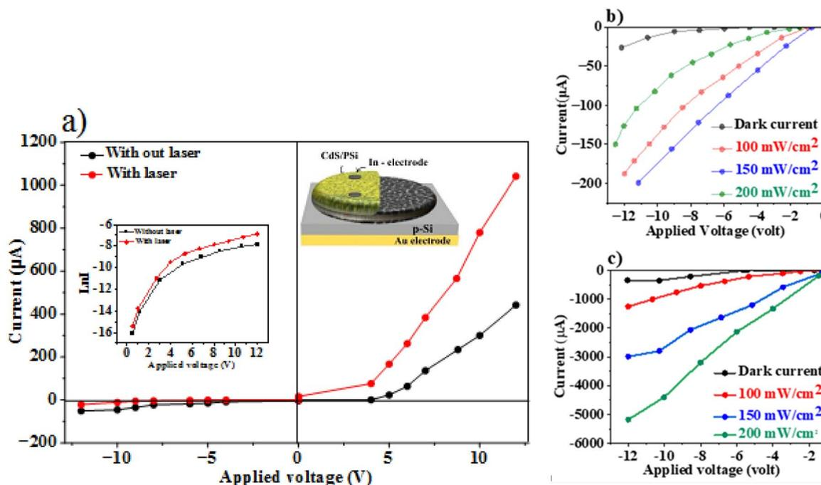
Fig. 4 (a) The profile of the  $I$ - $V$  characteristics, inset semi-logarithmic  $I$ - $V$  plot and a cross-sectional schematic design of the CdS/PSi photodetector, (b) illuminated  $I$ - $V$  characteristics of CdS/PSi photodetector prepared with laser, (c) illuminated  $I$ - $V$  characteristics of CdS/PSi photodetector prepared without laser illumination.
