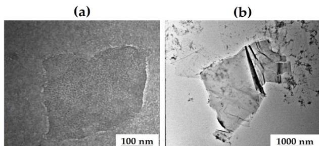
Fig. 1 TEM images of (a) pristine clay and (b) graphene sheet.
