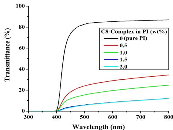
Fig. 12 UV-vis. Transmittances of PI hybrid films containing various C8-complex contents.
