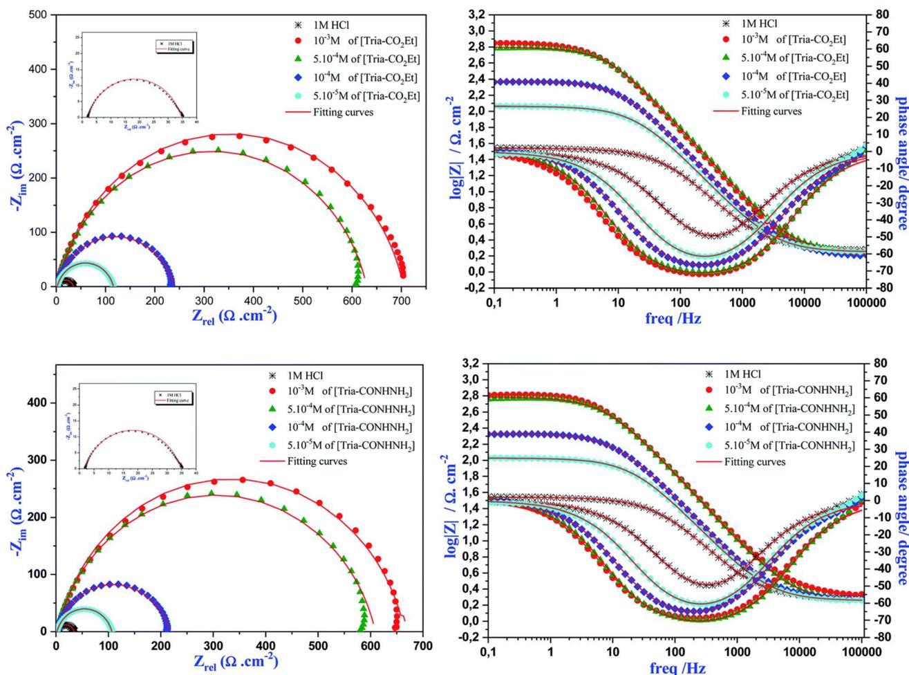
Fig. 19 Nyquist and Bode plots for mild steel in 1.0 M HCl with and without various [Tria-CO<sub>2</sub>Et] and [Tria-CONHNH<sub>2</sub>] concentrations, reproduced from ref. 56 with permission from [RSC] [RSC Adv., 2021, 11, 4147–4162] copyright 2021.
