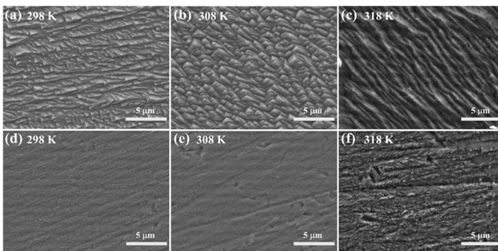
Fig. 25 FE-SEM micrographs of the X70 steel specimens immersed in 1 M HCl solution (a–c) without and (d–f) with 200 mg L<sup>-1</sup> GLE for 4 h at different temperatures, reproduced from ref. 70 with permission from [Elsevier] [*Corros. Sci.*, 2018, **133**, 6–16] copyright 2018.
