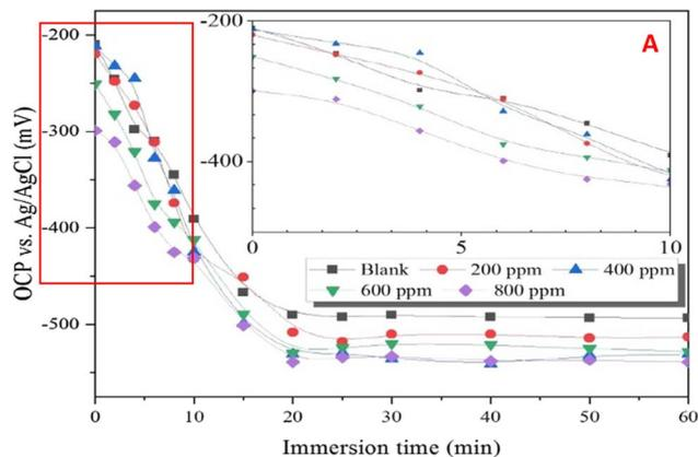
Fig. 18 The open circuit potential (OCP) variation with immersion time for mild steel exposed in uninhibited and inhibited 1 M HCl solution (Inhibitor; different quantities of *Ziziphora* leaves extract); inset shows the enlarged view of region 'A' marked in red colour, reproduce from ref. 54, with permission from [Elsevier] [*Constr. Build. Mater.*, 2020, 245, 118464] copyright 2020.
