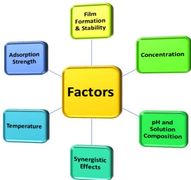
Fig. 12 Factors responsible for organic corrosion inhibitors.
