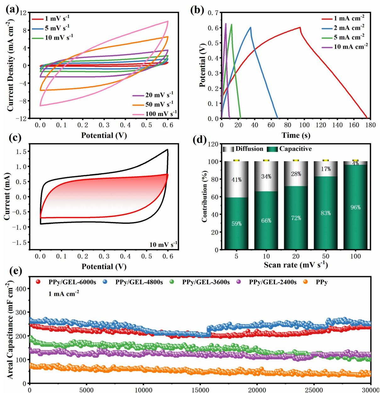
Fig. 5 (a) CV curves and (b) GCD curves for the PPy/GEL-4800s supercapacitor. (c) CV curve of PPy/GEL-4800s at 10 mV s<sup>-1</sup>. (d) Capacity contribution of PPy/GEL-4800s at different scan rates. (e) Cycling performance of the PPy/GEL device at a current of 1 mA cm<sup>-2</sup>.
