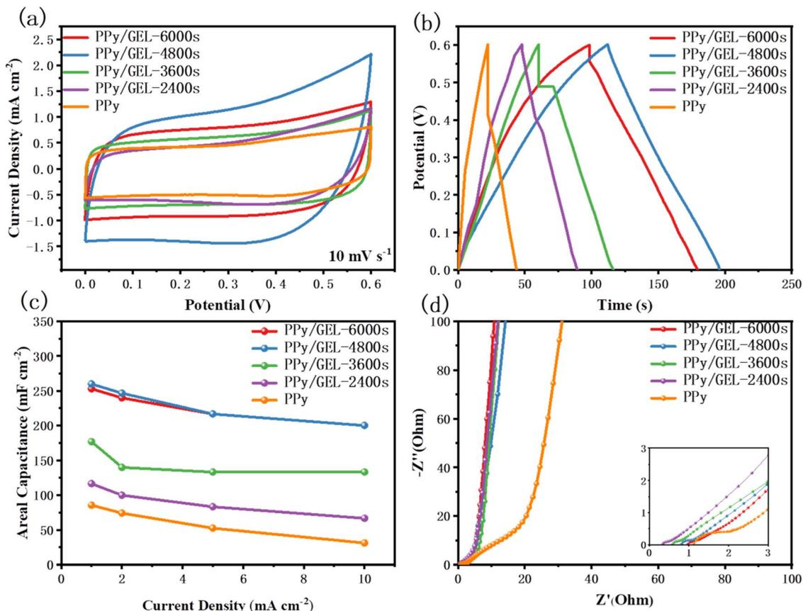
Fig. 4 (a) CV curves of pure PPy and various PPY/GEL SCs at  $10 \text{ mV s}^{-1}$ , (b) the second cycle GCD curves of pure PPy and various PPY/GEL SCs at  $1 \text{ mA cm}^{-2}$ , (c) areal capacitance of pure PPy and PPY/GEL SCs at various current densities ranging from 1 to  $10 \text{ mA cm}^{-2}$  and (d) Nyquist plots.
