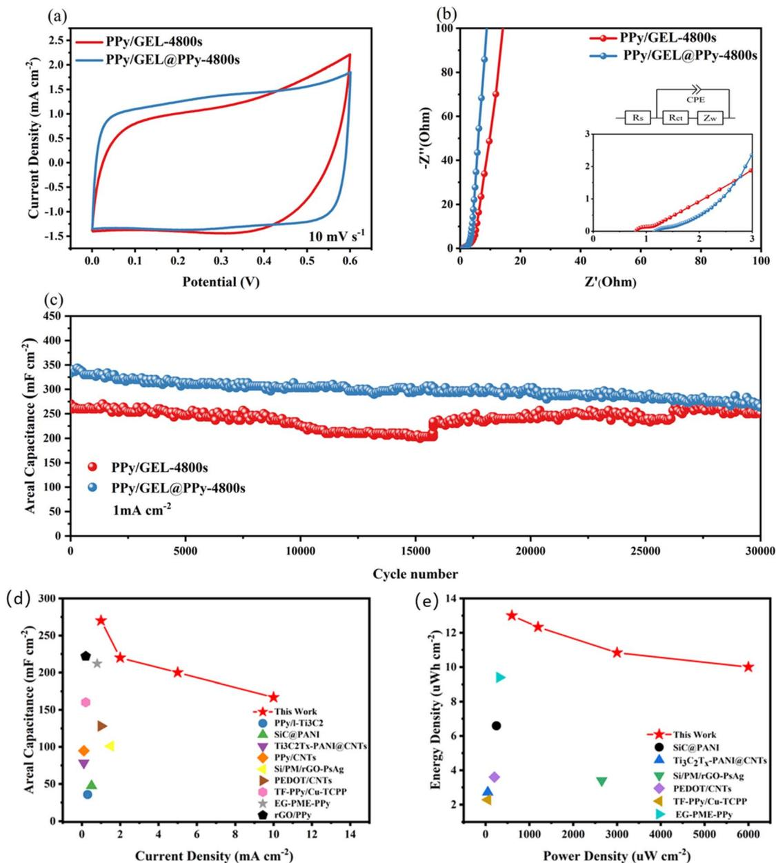
Fig. 7 Electrochemical properties of GelMA with or without Py. (a) CV curves. (b) Nyquist plot. (c) Stability tests of SC at current density of  $1 \text{ mA cm}^{-2}$ . (d) Areal capacitance in comparison with reported values. (e) Energy density in comparison with reported values.
