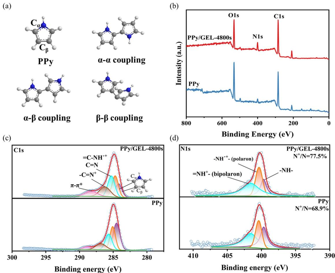
Fig. 3 (a) Three coupling methods ( $\alpha$ - $\alpha$ ,  $\alpha$ - $\beta$ ,  $\beta$ - $\beta$ ) of PPy. (b) XPS survey spectra of PPy/GEL and pure PPy. Fitted C 1s spectra of (c) PPy/GEL and pure PPy and (d) N 1s of PPy/GEL and pure PPy.
