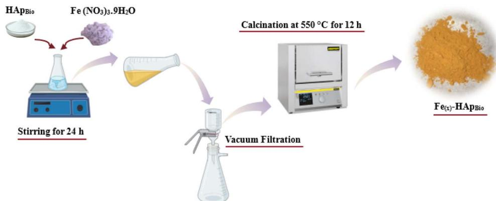
Fig. 2 Synthesis process of the Fe<sub>(x)</sub>-HAp<sub>Bio</sub> catalyst.
