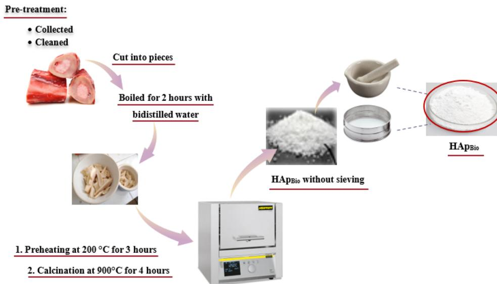
Fig. 1 Synthesis process of bio-hydroxyapatite (HAp<sub>Bio</sub>).
