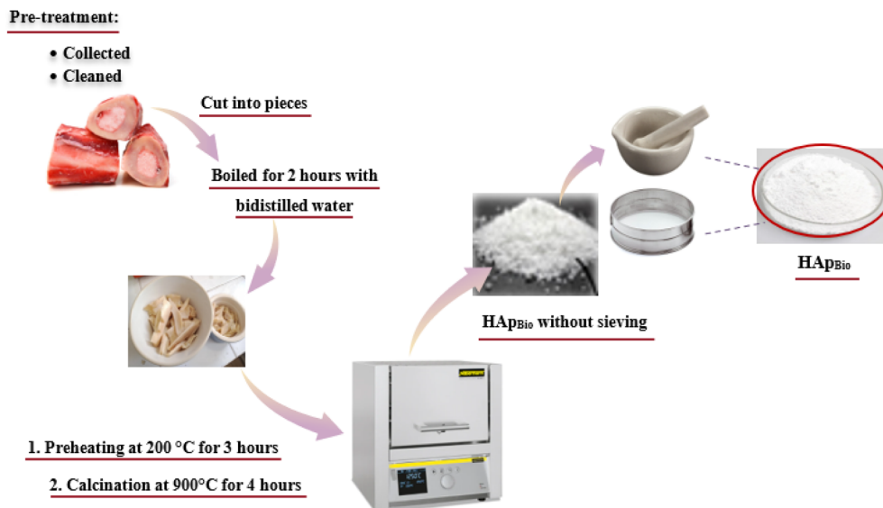
Fig. 1 Synthesis process of bio-hydroxyapatite (HAp Bio ).
