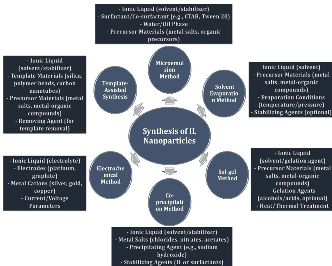
Fig. 3 Schematic representation of ionic liquids as nanoparticles and common methods of synthesis.
