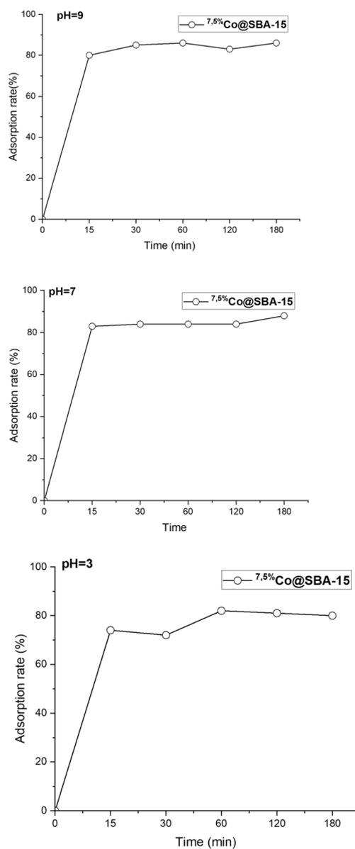
Fig. 10 Adsorption of tetracycline at different pH over 7.5%Co@SBA-15.
