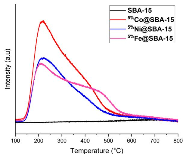
Fig. 5  $\text{NH}_3$ -TPD profile of  $5\% \text{Ni@SBA-15}$ ,  $5\% \text{Co@SBA-15}$  and  $5\% \text{Fe@SBA-15}$  plotted against the one of the pristine SBA-15 support.
