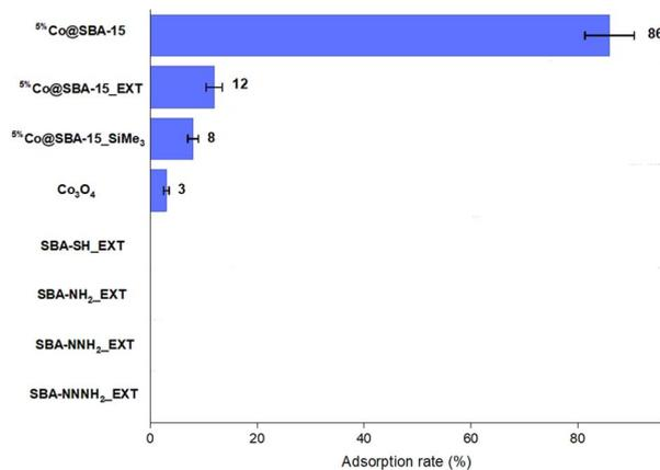
Fig. 7 Adsorption of tetracycline after  $t = 180$  min using various SBA-15-type materials (SBA-NH<sub>2</sub>\_EXT, SBA-NNH<sub>2</sub>\_EXT, SBA-NNNH<sub>2</sub>\_EXT, SBA-SH\_EXT),  $\text{Co}_3\text{O}_4$ ,  $^{5\%}\text{Co@SBA-15\_EXT}$ ,  $^{5\%}\text{Co@SBA-15}$  and  $^{5\%}\text{Co@SBA-15\_SiMe}_3$ .
