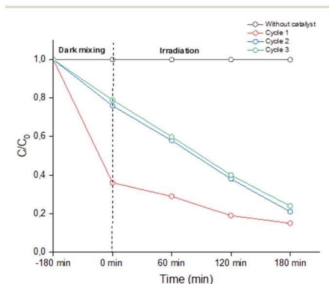
Fig. 13 Recycling photocatalytic experiments of tetracycline ( $C = 10^{-3}$  mol  $\text{L}^{-1}$ ) degradation with  $^{7.5\%}\text{Co@SBA-15}$  assuming an adsorption equilibrium after 3 hours.
