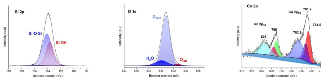
Fig. 4 XPS spectra of the Si 2p, O 1s, and Co 2p peaks of  $5\% \text{Co@SBA-15}$ .
