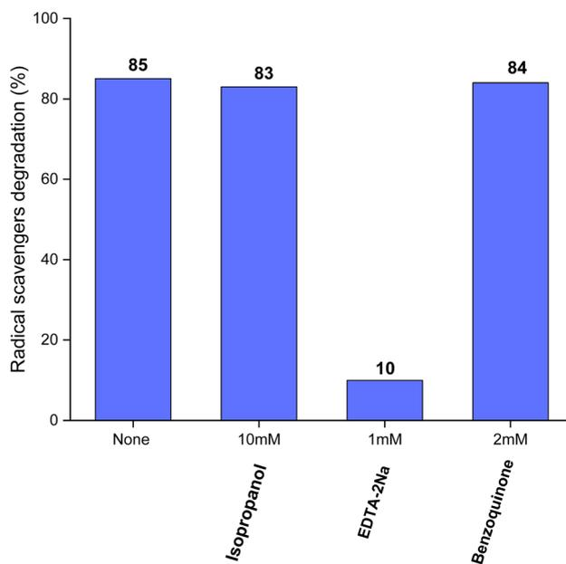
Fig. 12 Visible-light photocatalytic activity of  $^{7.5\%}\text{Co@SBA-15}$  against tetracycline ( $C = 10^{-3} \text{ mol L}^{-1}$ ) assuming an equilibrium of adsorption after 3 hours and the corresponding radical scavenging tests.
