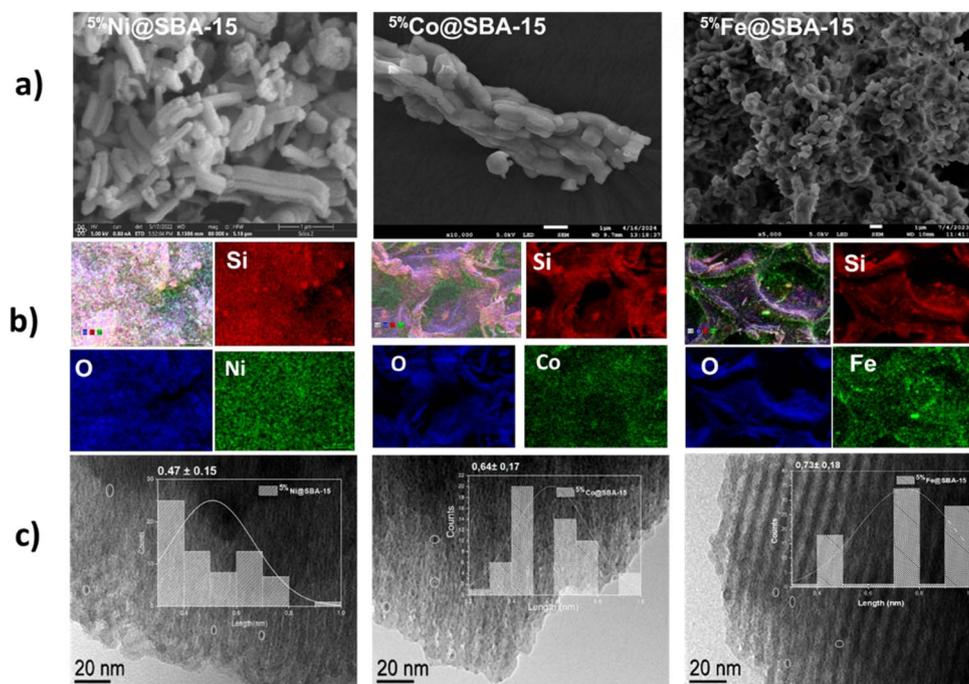
Fig. 3 Scanning and transmission electronic microscopy of  $5\% \text{Ni@SBA-15}$ ,  $5\% \text{Co@SBA-15}$  and  $5\% \text{Fe@SBA-15}$ . (a) SEM, (b) EDX mapping of oxygen, silicon and the metal for each material, and (c) TEM images and histograms of the size distribution of the corresponding metal nanoparticles.
