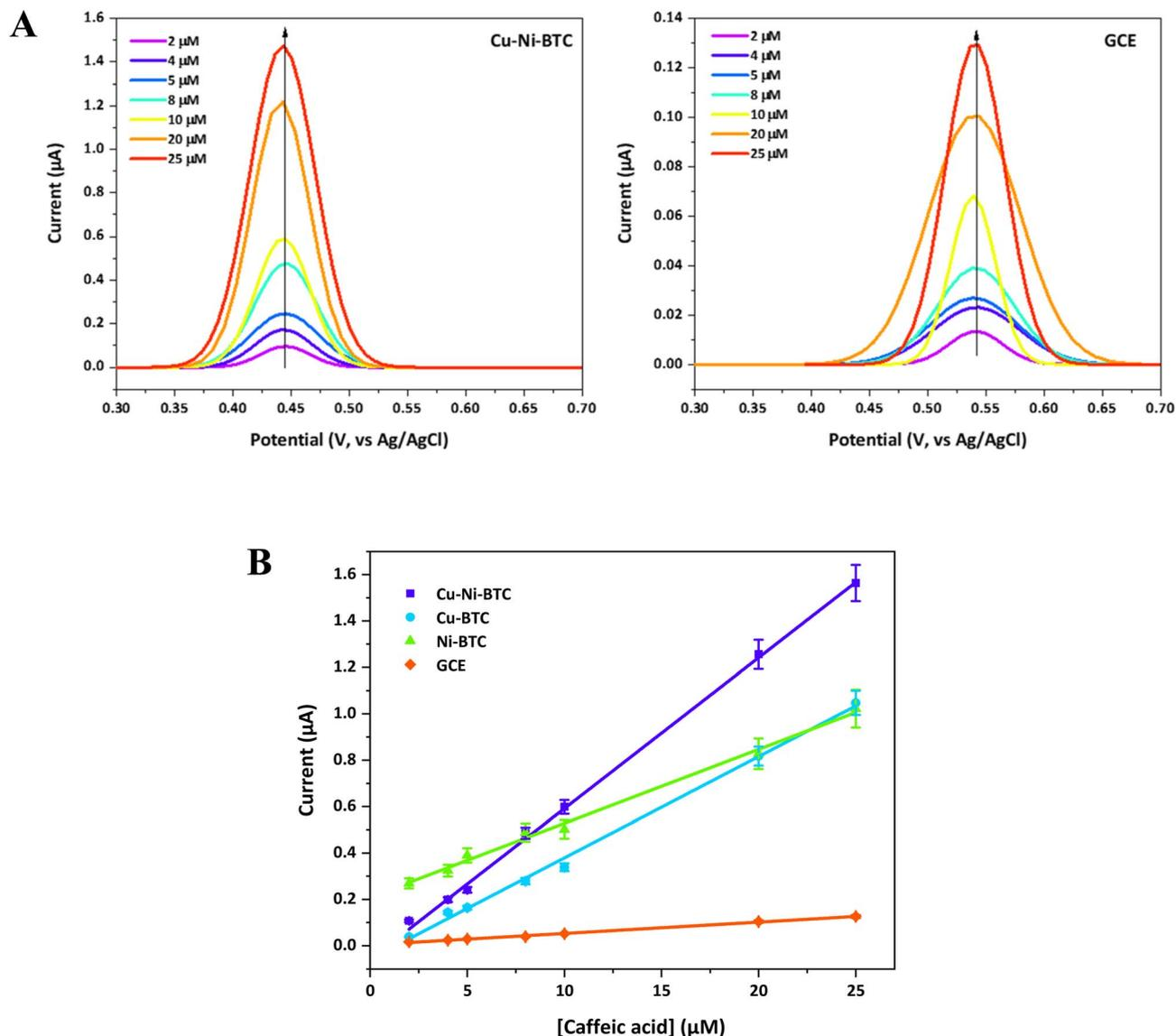
Fig. 7 Detection of caffeic acid using the electrodeposited Cu,Ni-BTC film. (A) DPV curves recorded on the electrodeposited Cu,Ni-BTC film and bare GCE in PBS (pH 3) containing caffeic acid at different concentrations (2–25 μM). (B) Calibration curves; values represent mean  $\pm$  SD ( $n = 3$ ).
