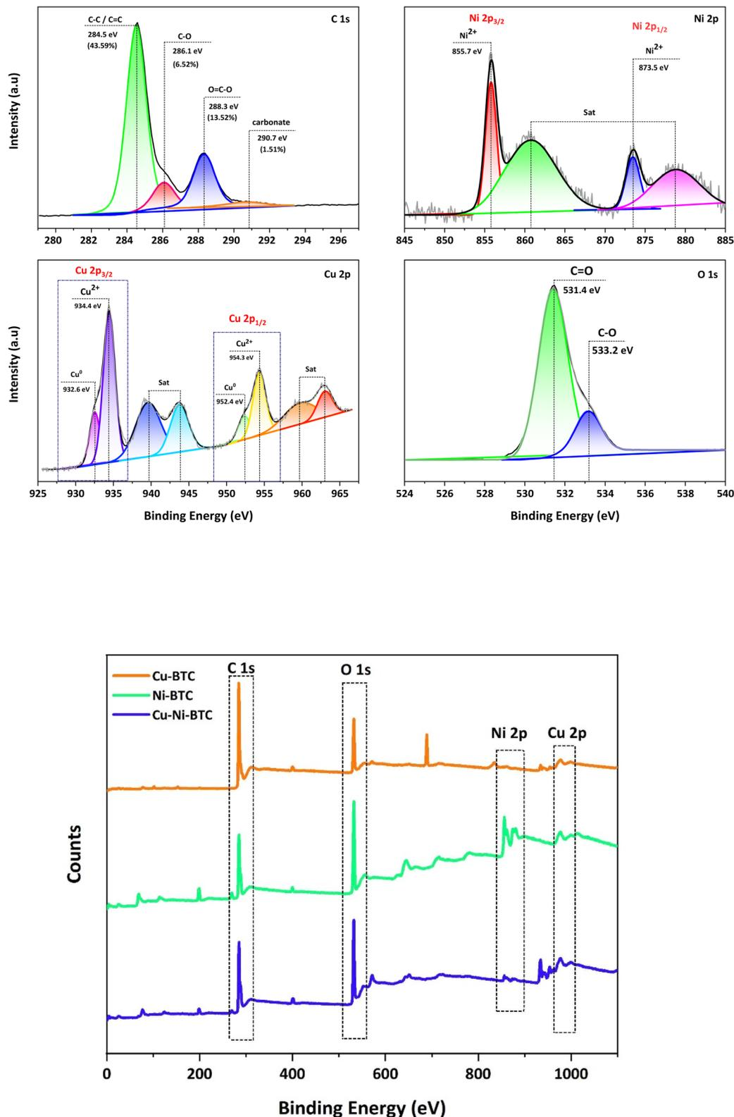
Fig. 2 XPS analysis of the electrodeposited Cu,Ni-BTC film. The survey spectrum and high-resolution C 1s, O 1s, Cu 2p, and Ni 2p spectra were recorded using monochromatic Al-K (1486.6 eV).
