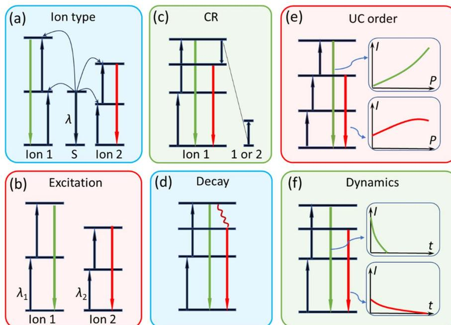
Fig. 4 Schematic diagrams illustrating the color change of Ln UCNCs based on different mechanisms.
