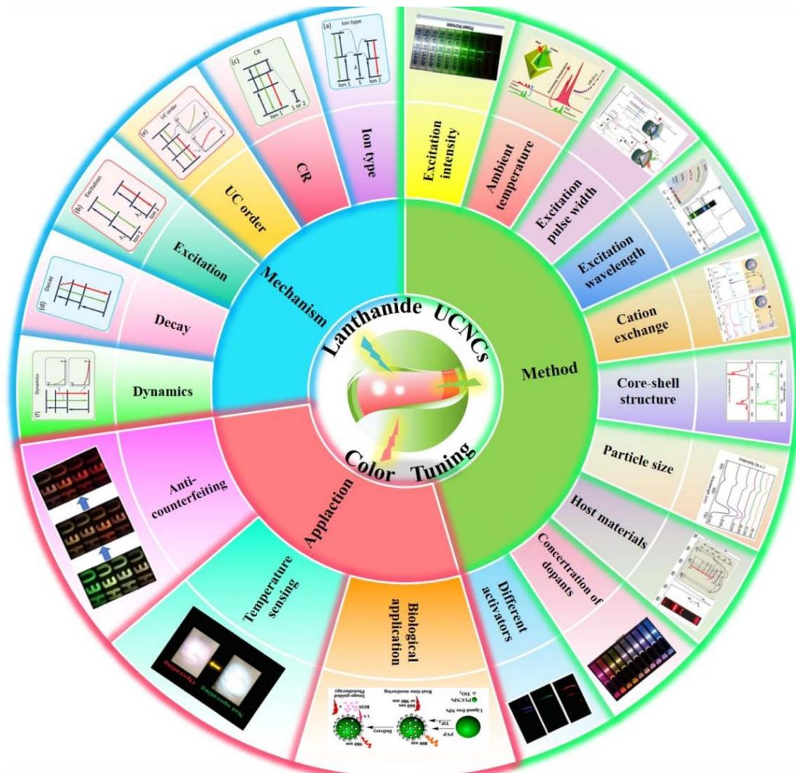
Fig. 1 Overview of Ln UCNCs color tuning, showing the main mechanisms, tuning strategies, and applications of the color-tunable UCNCs.
