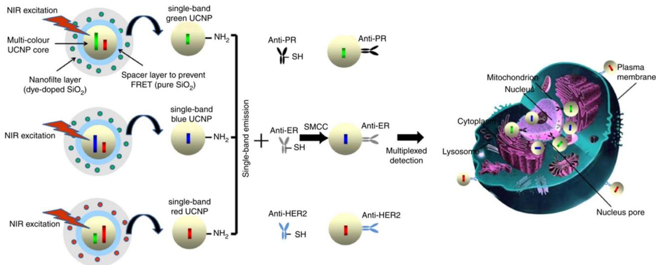
Fig. 17 Schematic diagram of single-band UCNCs fabrication for multiplexed detection. Surface amino modifications formed the R/G/B single-band UCNCs, for multiplexed *in situ* molecular mapping of breast cancer. Reproduced with permission.<sup>171</sup> Copyright 2015, Springer Nature.
