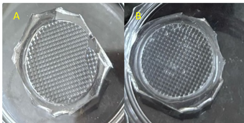
Fig. 4 Damage caused to device during peeling from un-silanized molds. (A&B) Image of device torn and structure damage occurred during peeling.
