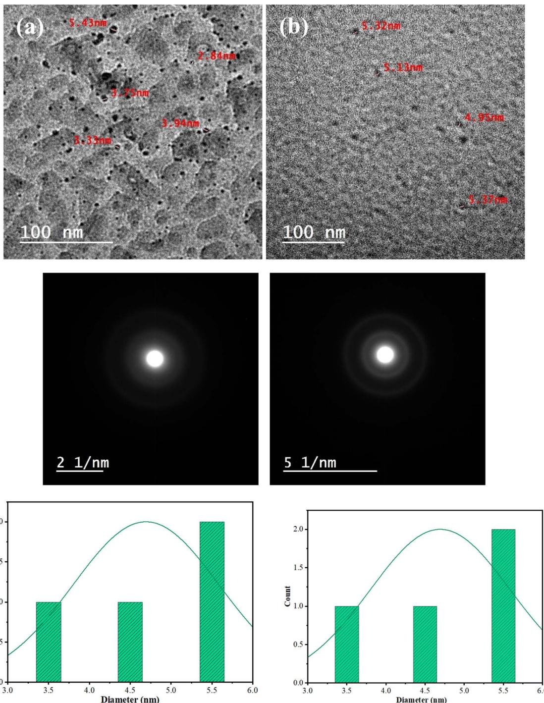
Fig. 4 TEM analysis and particle size histogram with SAED for (a) Cu-Fe<sub>3</sub>O<sub>4</sub>/CDs and (b) Al/Cu-Fe<sub>3</sub>O<sub>4</sub>/CDs.
