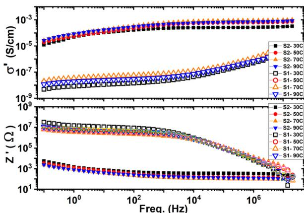
Fig. 8 Conductivity,  $\sigma'$ , and Impedance,  $Z'$ , as frequency functions of S1: Cu- $\text{Fe}_3\text{O}_4/\text{CDs}$  and S2: Al/Cu- $\text{Fe}_3\text{O}_4/\text{CDs}$  at different temperatures.
