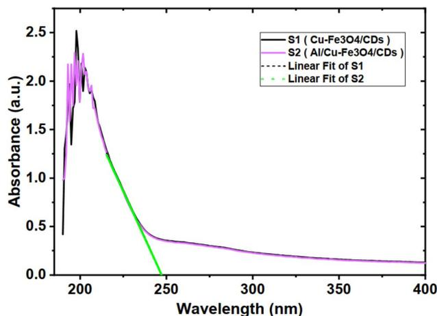
Fig. 6 UV-vis spectra of Cu-Fe<sub>3</sub>O<sub>4</sub>/CDs and Al/Cu-Fe<sub>3</sub>O<sub>4</sub>/CDs.
