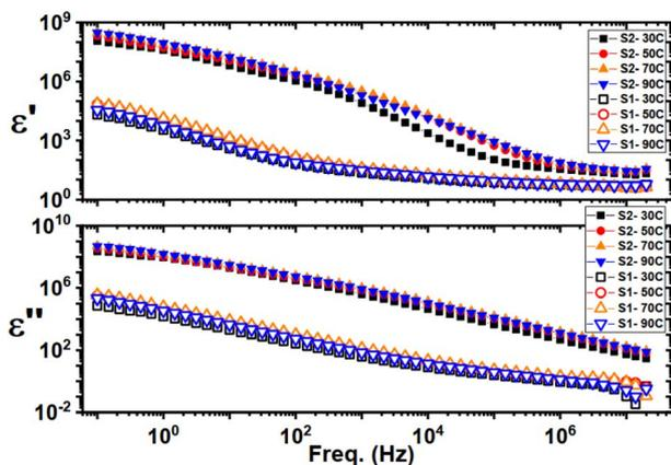
Fig. 7 Permittivity,  $\epsilon'$ , and Loss,  $\epsilon''$ , as frequency functions of S1: Cu- $\text{Fe}_3\text{O}_4/\text{CDs}$  and S2: Al/Cu- $\text{Fe}_3\text{O}_4/\text{CDs}$  at different temperatures.
