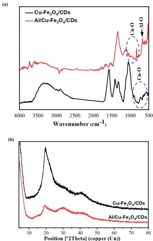
Fig. 5 FTIR spectra (a) and XRD (b) of Cu-Fe<sub>3</sub>O<sub>4</sub>/CDs and Al/Cu-Fe<sub>3</sub>O<sub>4</sub>/CDs.
