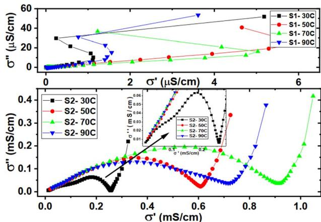
Fig. 10 Cole–Cole plot of conductivity for S1: Cu–Fe<sub>3</sub>O<sub>4</sub>/CDs and S2: Al/Cu–Fe<sub>3</sub>O<sub>4</sub>/CDs at different temperatures.
