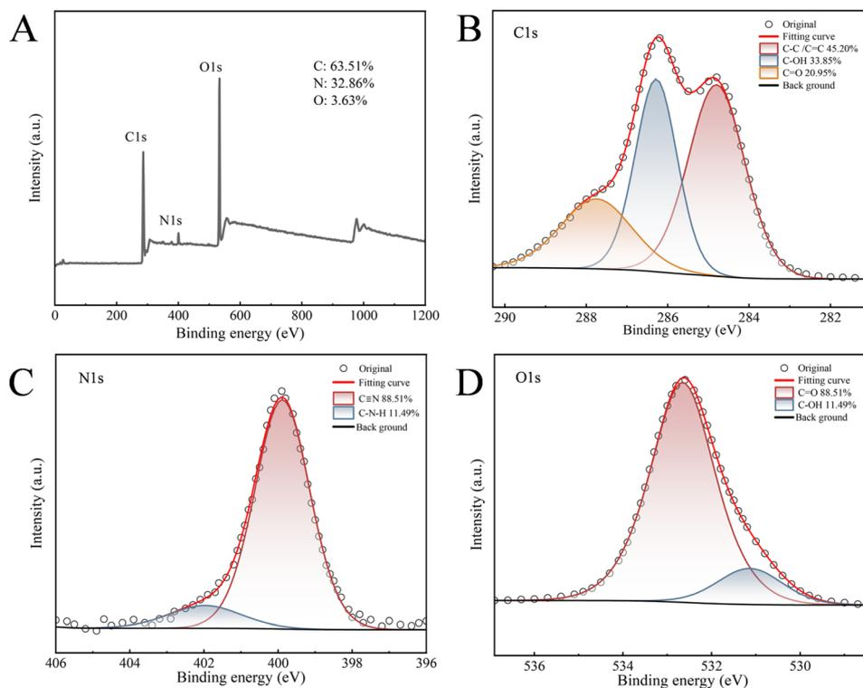
Fig. 3 XPS analysis of B-CQDs: (A) full survey spectrum; high-resolution spectra of (B) C 1s, (C) O 1s, and (D) N 1s.
