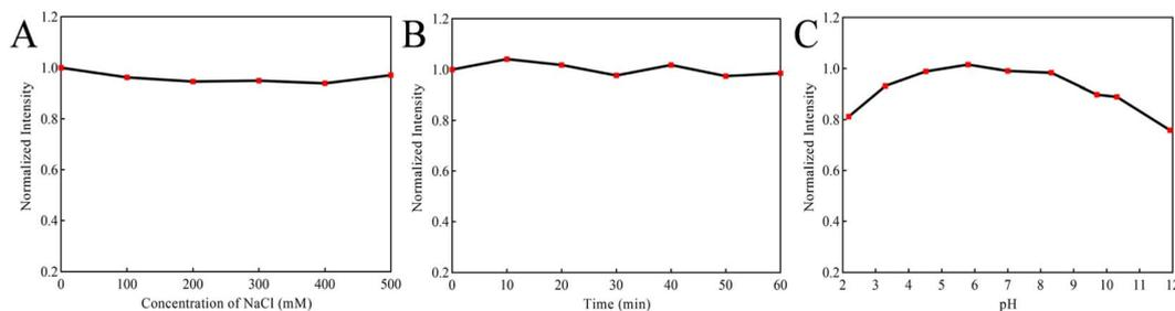
Fig. 5 Stability evaluation of B-CQDs: (A) Effect of ionic strength (NaCl concentration: 0–500 mM) on fluorescence intensity; (B) photostability under continuous 365 nm UV irradiation; (C) pH dependence of fluorescence intensity (pH range: 2.18–11.92).
