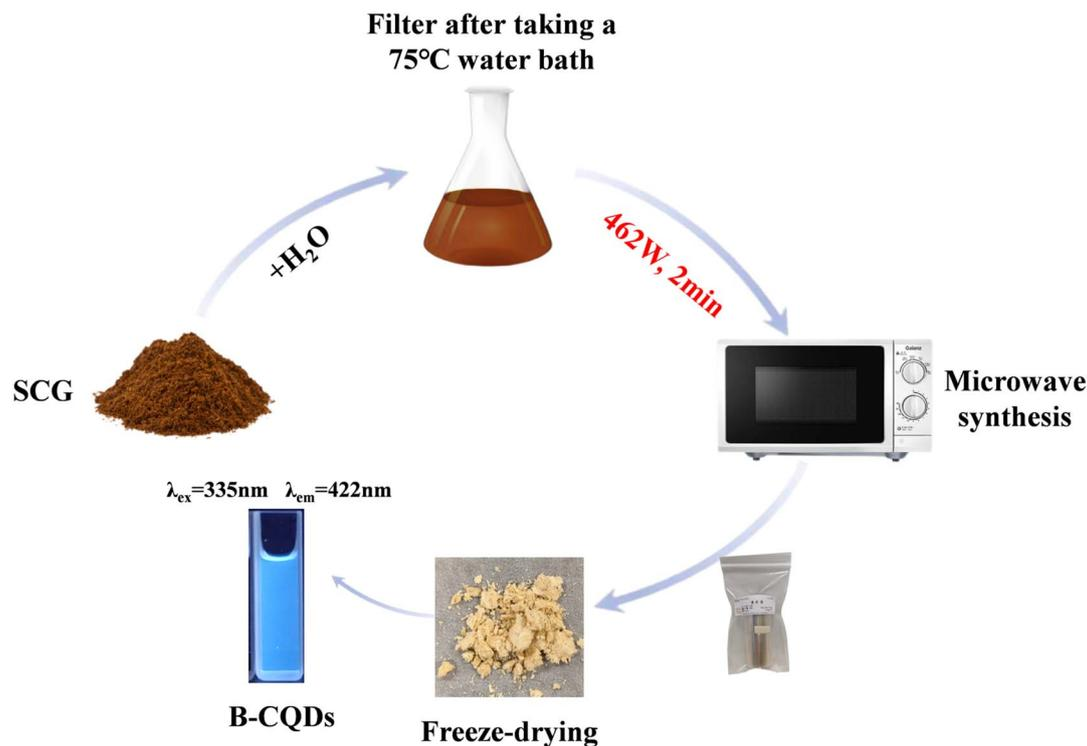
Fig. 1 Schematic illustration of the synthesis procedure for B-CQDs.
