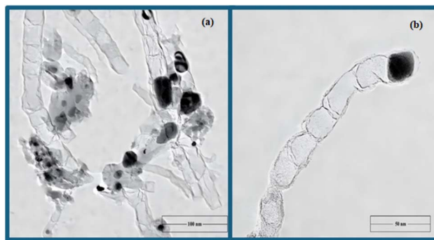
Fig. 7 TEM analysis of the CNT-AMP adsorbent, (a) scale: 100 nm, (b) scale: 50 nm.
