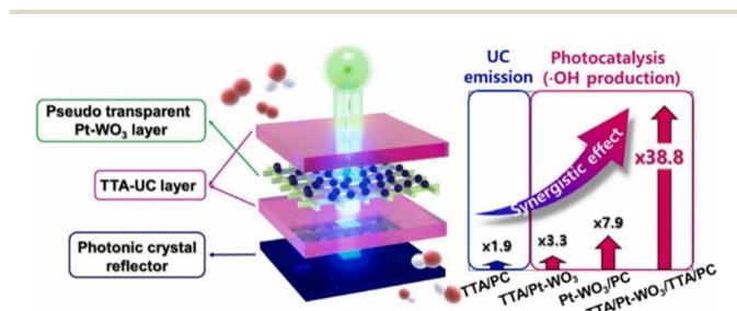
Fig. 5 Schematic illustration of the TTA/Pt-WO<sub>3</sub>/TTA/Photonic crystal multi-layered sub-bandgap photocatalytic reactor. UC emission enhancement is analyzed compared the full TTA-UC system, while the  $\cdot\text{OH}$  generation efficiency for photooxidation of pollutants is compared to that of the Pt-WO<sub>3</sub> layer in each combination. Reproduced from Cho *et al.*,<sup>102</sup> copyright 2024 Elsevier B.V.
