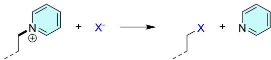
Scheme 4 Schematic representation of the halide-assisted cleavage of the N1–C2 bond resembling S_N2 process and liberating neutral pyridine.
