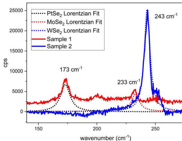
Fig. 3 Raman spectra of Sample 1 (1L MoSe<sub>2</sub> + 2L PtSe<sub>2</sub>, red) and Sample 2 (3L WSe<sub>2</sub>, blue) together with their Lorentzian fits (dotted lines). The spectra were background corrected with respect to the Mica reference. For PtSe<sub>2</sub>, there is a second peak around 200 cm<sup>-1</sup> that should also be considered in the fits, its intensity is weak in agreement with the 2L thickness of PtSe<sub>2</sub>.<sup>52</sup>
