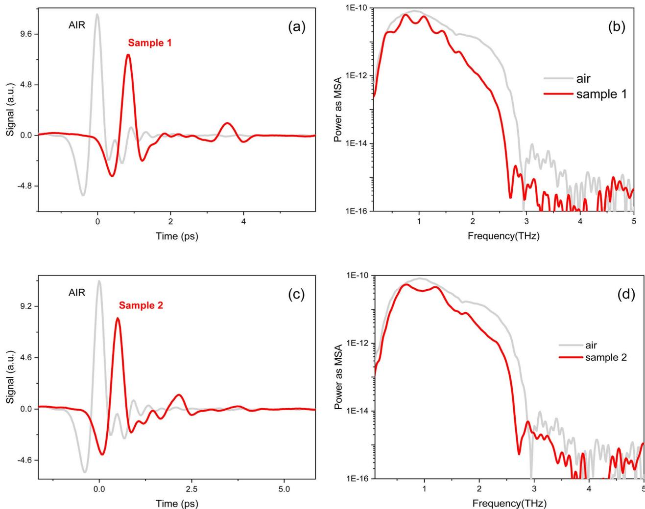
Fig. 10 (a) THz time-domain profiles and (b) corresponding frequency-domain spectra of air reference and Sample 1 (1L MoSe<sub>2</sub> + 2L PtSe<sub>2</sub>) and (c) THz time-domain profiles and (d) corresponding frequency domain spectra of reference air and Sample 2 (3L WSe<sub>2</sub>).
