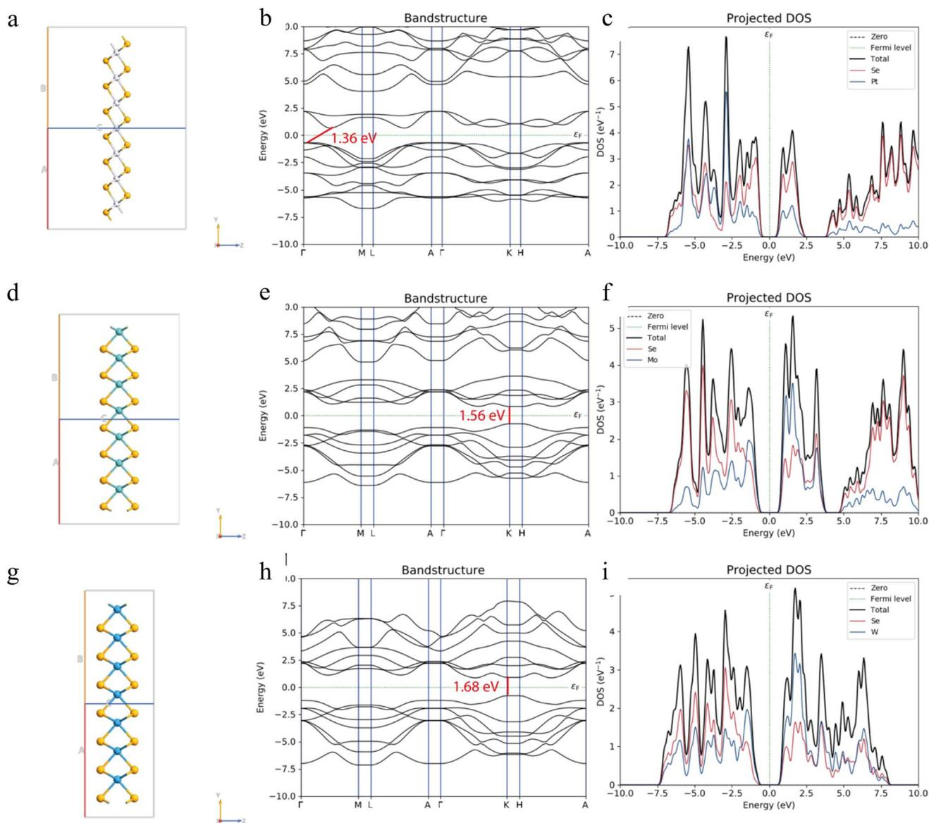
Fig. 7 Electronic properties of PtSe<sub>2</sub>, MoSe<sub>2</sub>, and WSe<sub>2</sub> as single layer. (a) Schematic representation of PtSe<sub>2</sub>, (b) its respective bandstructure, and (c) its PDOS. (d) Molecular structure of MoSe<sub>2</sub>, (e) its respective bandstructure and (f) its PDOS. (g) Atomistic arrangement of WSe<sub>2</sub>, (h) its respective bandstructure, and (i) its PDOS.
