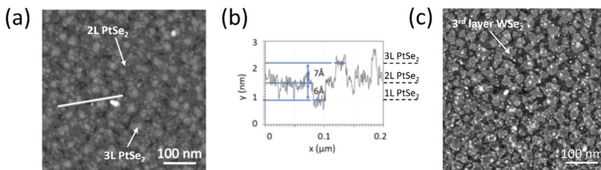
**Fig. 6** (a) 500 × 500 nm<sup>2</sup> AFM image of Sample 1 (1L MoSe<sub>2</sub> + 2L PtSe<sub>2</sub>) showing almost 100% coverage. (b) Height profile recorded along the white line in (a) showing the vdW stacking. (c) 500 × 500 nm<sup>2</sup> AFM image of Sample 2 (3L WSe<sub>2</sub>).
