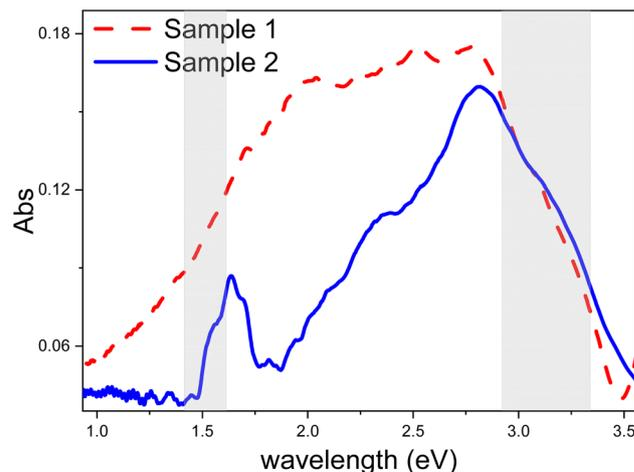
Fig. 2 UV-Vis spectra of Sample 1 (1L MoSe<sub>2</sub> + 2L PtSe<sub>2</sub>) (dashed red line) and Sample 2 (3L WSe<sub>2</sub>) (solid blue line). The gray areas represent the excitation wavelengths of 800 nm (1.55 eV) and 400 nm (3.10 eV) with their corresponding bandwidths for TRTS studies.
