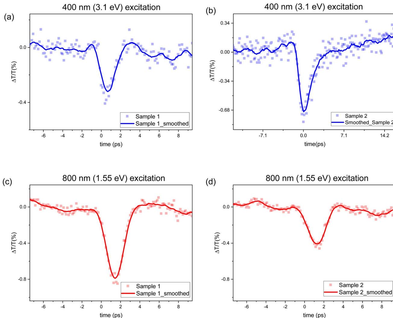
Fig. 12 Differential THz transmission,  $\Delta T/T_0$ , of (a) Sample 1 and (b) Sample 2 as a function of pump-probe delay recorded at a fluence of  $195 \mu\text{J cm}^{-2}$  for 400 nm excitation and  $\Delta T/T_0$  of (c) Sample 1 and (d) Sample 2 at a fluence of  $255 \mu\text{J cm}^{-2}$  for 800 nm excitation. (The solid lines are 20-point Savitzky-Golay averaging).
