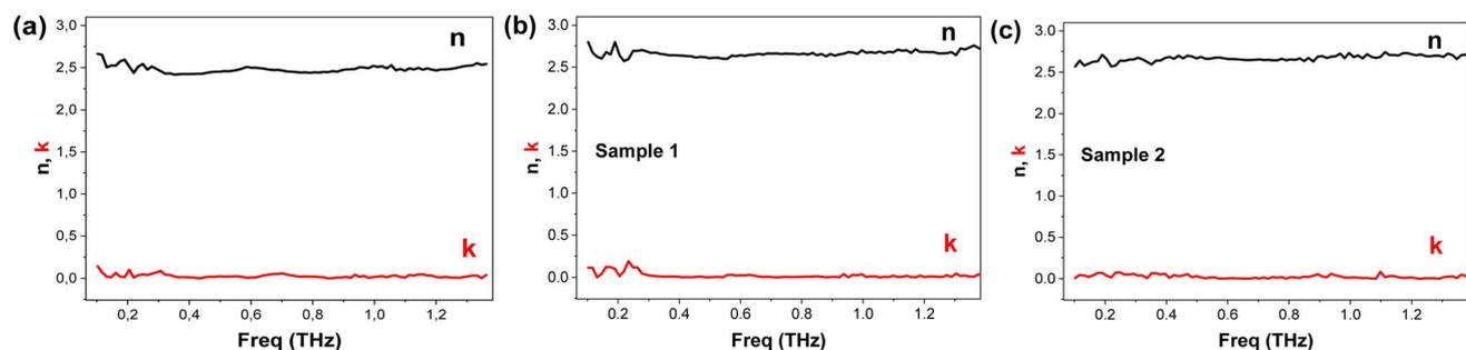
Fig. 11 Refractive index ( $n$ ) and extinction coefficient ( $k$ ) of (a) mica substrate and (b) Sample 1 (mica + 1L MoSe<sub>2</sub> + 2L PtSe<sub>2</sub>), (c) Sample 2 (mica + 3L WSe<sub>2</sub>).
