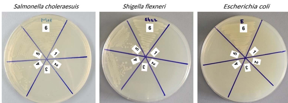
Fig. 5 MHA agar plates showing the MIC/MBC of S. choleraesuis , S. flexneri and E. coli upon treatment with ZnMoVS 4 NPs (1: 16 mg mL -1 , 2: 8 mg mL -1 , 3: 4 mg mL -1 , 4: 2 mg mL -1 , 5: 1 mg mL -1 , 6: untreated bacteria).
