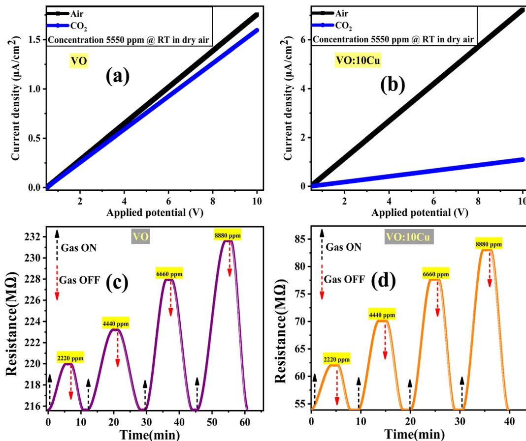
Fig. 6 (a) and (b) *I-V* characteristic curves, and (c) and (d) dynamic response for pure V<sub>2</sub>O<sub>5</sub>, and 10 at% Cu-V<sub>2</sub>O<sub>5</sub>, respectively.
