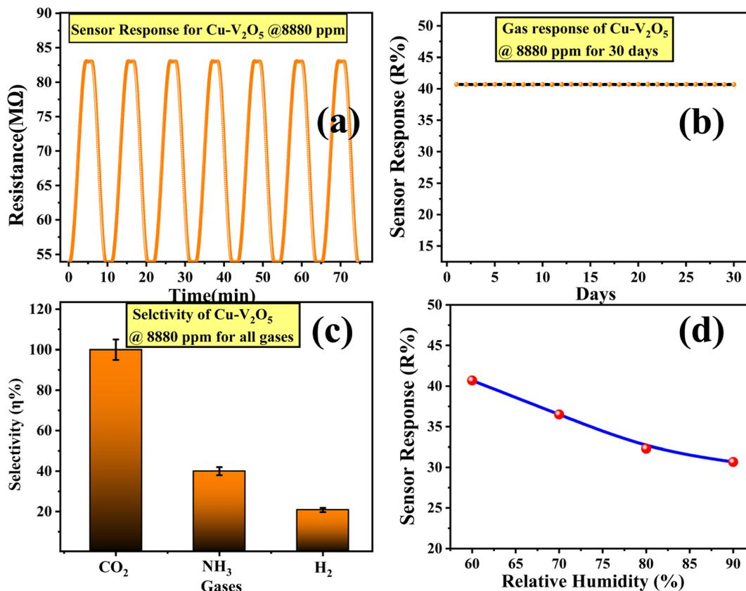
Fig. 8 (a) Repeatability, (b) stability, (c) selectivity for several gases at 8880 ppm concentration, RT, and 60% RH, and (d) sensor response vs. relative humidity for 10 at% Cu-doped V<sub>2</sub>O<sub>5</sub> sensor.
