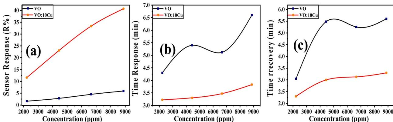
Fig. 7 (a) Sensor response, (b) response time, (c) recovery time vs. gas concentration for pure V<sub>2</sub>O<sub>5</sub> and 10 at% Cu-V<sub>2</sub>O<sub>5</sub>, respectively.
