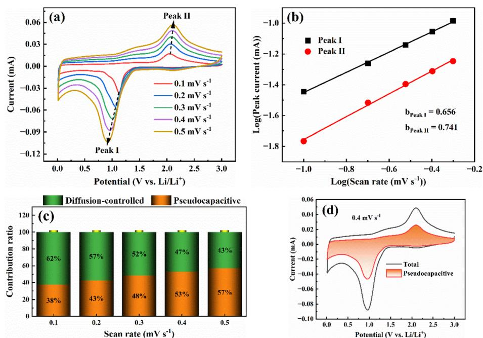
Fig. 6 (a) CV plots of CoO/MC electrode at different scanning rates; (b)  $\log i$  vs.  $\log v$  plot for CoO/MC electrode; (c) contribution ratio of the capacitance-controlled and diffusion-controlled charge versus scanning rate; (d) Separation of the capacitive and diffusion currents in CoO/MC at a scanning rate of 0.4  $\text{mV s}^{-1}$ .
