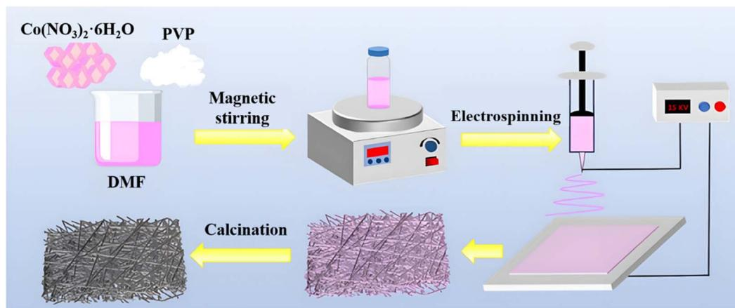
Fig. 1 Illustration of preparing CoO/C composite nanofiber.
