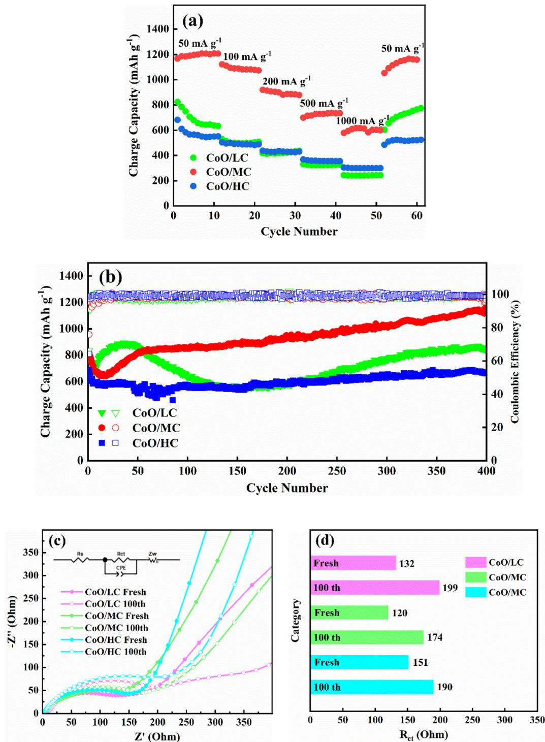
Fig. 7 (a) Rate performances of CoO/LC, CoO/MC, CoO/HC. (b) Cyclic performance of CoO/LC, CoO/MC, CoO/HC at 100 mA g<sup>-1</sup>. (c) The EIS spectra for the fresh and cycled electrodes of CoO/LC, CoO/MC, CoO/HC. (d) The corresponding R<sub>ct</sub> values for the fresh and cycled electrodes of CoO/LC, CoO/MC, CoO/HC.
