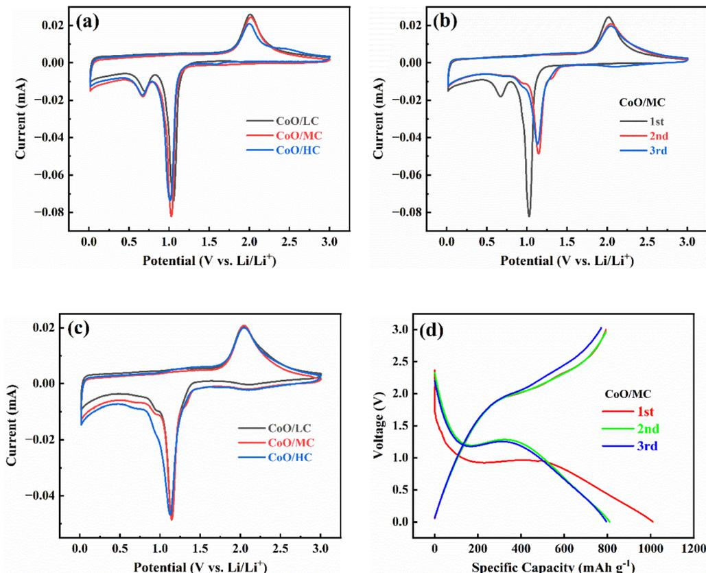
Fig. 5 (a) The first CV profiles for CoO/LC, CoO/MC, CoO/HC electrodes at  $0.1 \text{ mV s}^{-1}$ . (b) Evolution of CVs obtained by cycling CoO/MC electrode at  $0.1 \text{ mV s}^{-1}$ . (c) The third CV profiles for CoO/LC, CoO/MC, CoO/HC electrodes at  $0.1 \text{ mV s}^{-1}$ . (d) Evolution of galvanostatic charge/discharge profiles obtained by cycling CoO/MC electrode at  $100 \text{ mA g}^{-1}$ .
