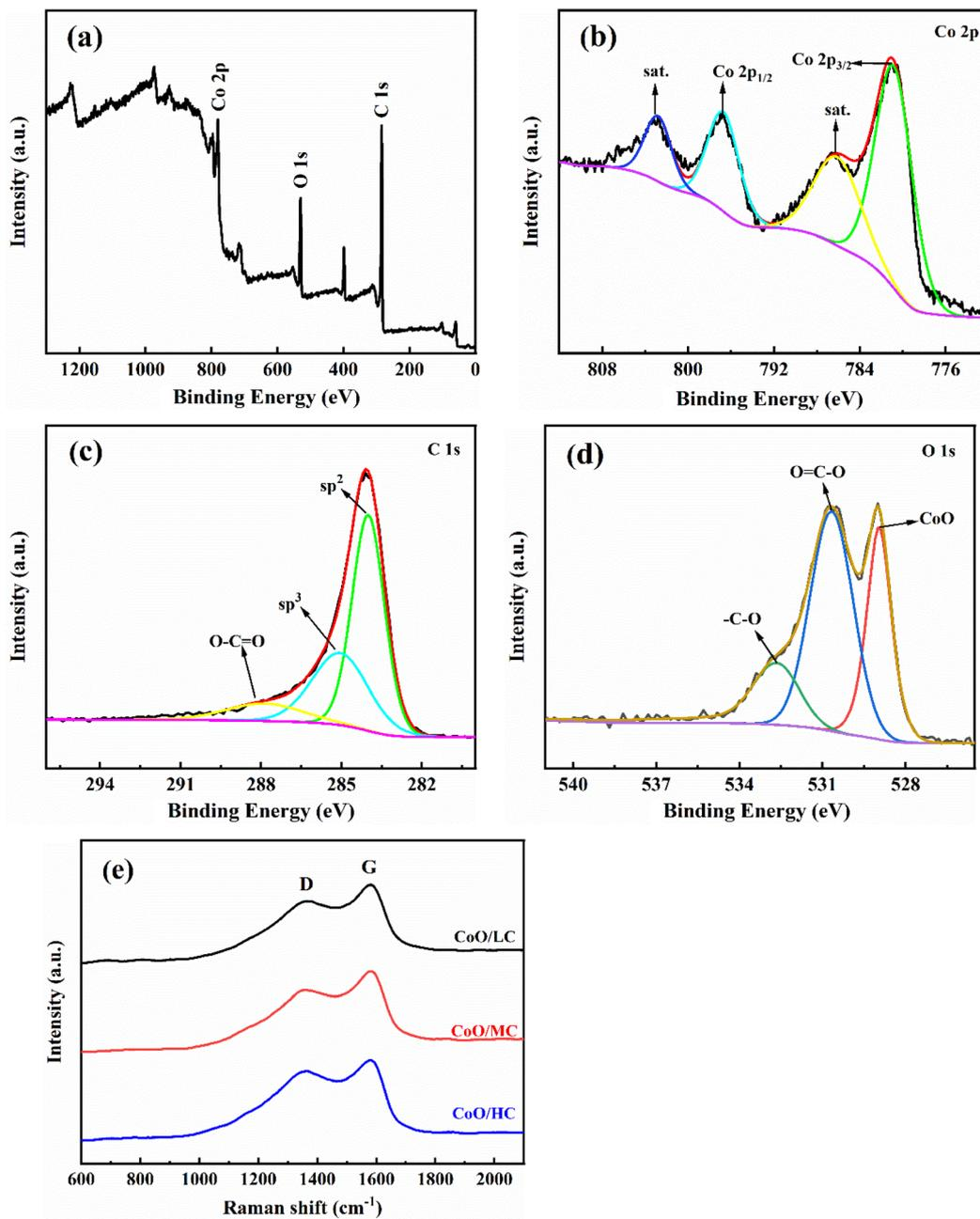
Fig. 4 (a) The full XPS spectra of CoO/MC sample; (b) Co 2p spectrum of CoO/MC sample; (c) C 1s spectrum of CoO/MC sample; (d) O 1s spectrum of CoO/MC sample; (e) the Raman spectra of three CoO/C samples.
