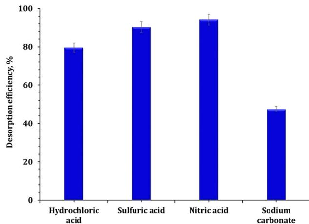
Fig. 12 The desorption efficiency from the loaded adsorbent.
