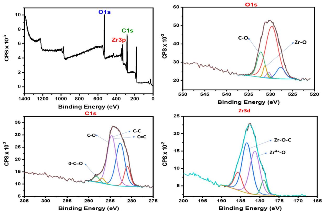
Fig. 4 XPS analyses of the applied Zr-GA adsorbent.
