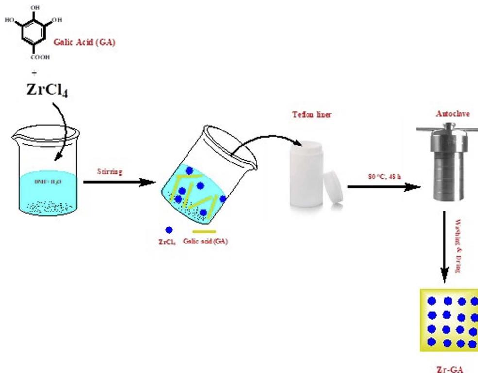
Fig. 1 The synthetic pathway for the adsorbent preparation.
