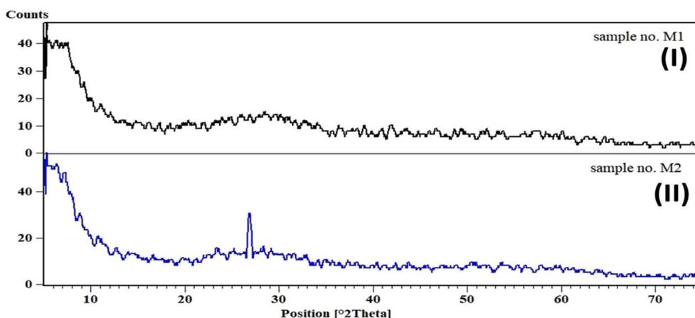
Fig. 2 XRD pattern of the gallic acid (I), and the Zr-GA (II) adsorbent.
