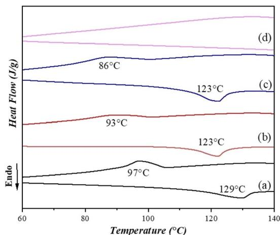
Fig. 7 DSC heat flow curves through the cycle of heating-cooling for TPS/PVA with different CA contents: (a) TC0, (b) TC10, (c) TC15, and (d) TC20.
