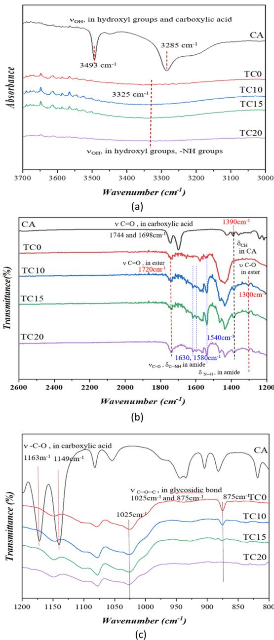
Fig. 2 ATR-FT/IR spectra of (a) the 3700–3000 cm<sup>-1</sup> region, (b) the 2600–1200 cm<sup>-1</sup> region, and (c) the 1200–800 cm<sup>-1</sup> region.
