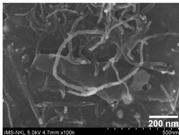
Fig. 3 SEM image of Gr-CNT-AgNP hybrid material.
