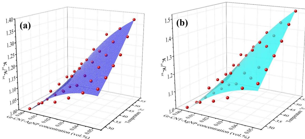
**Fig. 12** Thermal conductivity ratio of ternary hybrid nanofluids *versus* Gr-CNT-AgNP concentrations and temperatures (a) water-based and (b) EG-based ternary hybrid nanofluids. The points represent experimental values, whereas the surfaces are derived from the fitting function (3).
