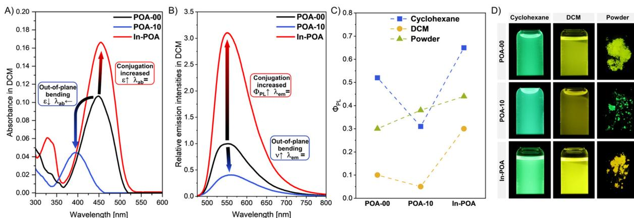
**Fig. 6** Selected display of the photophysical properties of compounds **POA-00**, **POA-10**, and **In-POA**: (A) UV/Vis spectra in DCM (15  $\mu$ M); (B) photoluminescence spectra in DCM (15  $\mu$ M) relative to **POA-00**; (C) absolute photoluminescence quantum yields  $\Phi_{PL}$  in cyclohexane, DCM, and as powders; (D) photographs of the three compounds in cyclohexane (left column), in DCM (centred column), and as powders (right column) under UV-light (365 nm).
