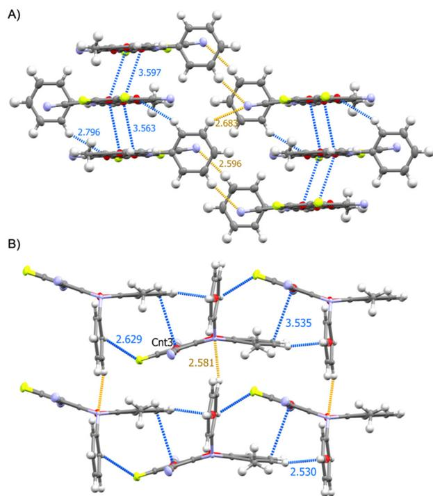
**Fig. 2** Excerpt of the crystal packings of (A) **POA-1'0** and (B) **POA-10**, showcasing the formation of (A)  $\pi$  stacked arrays with oxygen-driven hydrogen bonds between dimeric structures (blue lines) interconnected by nitrile-mediated hydrogen bonds (orange lines); (B) brick-like formation of trimeric layers with offset  $\pi\cdots\pi$  contacts (blue), interconnected by nitrogen-driven hydrogen bonds (orange lines). The displacement ellipsoids are displayed at 50% probability levels.
