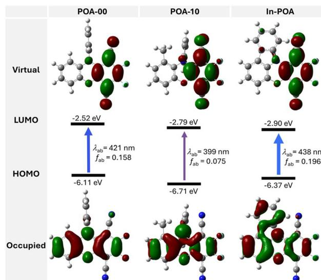
**Fig. 5** Calculated optimized geometries in the  $S_0$  states with the corresponding virtual and occupied natural transition orbital (NTO) pairs, energies of the HOMOs and LUMOs, as well as calculated absorption wavelengths  $\lambda_{\text{ab}}$  and oscillator strengths  $f_{\text{ab}}$  (calculated using TD-PBE0/TZVP) for compounds **POA-00**, **POA-10**, and **In-POA**.
