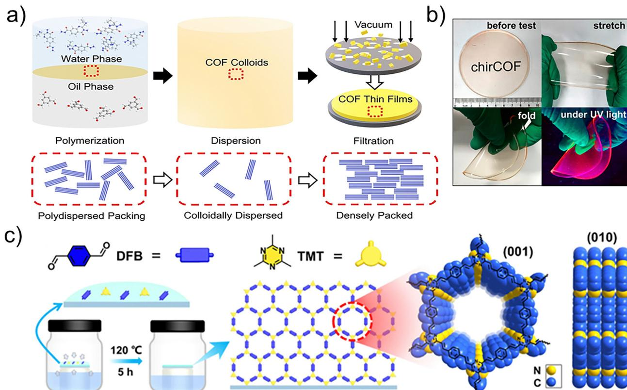
Fig. 6 Preparation methods for COF films. (a) Schematic illustration of the fabrication of self-standing chiral COF Films via a polymerization–dispersion–filtration sequence.<sup>59</sup> (b) Dispersed COF NS into polydimethylsiloxane (PDMS) matrix to obtain highly transparent, large size, and flexible films.<sup>54</sup> (c) Preparation of COF films via vapor-assisted epitaxial methods.<sup>58</sup>
