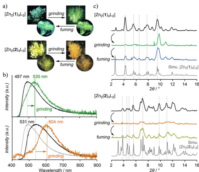
**Fig. 5** (a) The appearance of before and after mechanical stimulation. (b) Normalized solid-state emission spectra: (top) before (black line) and after (green line) of  $[\text{Zn}_2(\mathbf{1})_4\text{L}_2]$ ; (bottom) before (black line) and after (orange line) of  $[\text{Zn}_2(\mathbf{2})_4\text{L}_2]$  with  $[\text{Zn}_2(\mathbf{1})_4\text{L}_2]$  (gray line). (c) pXRD patterns of grinding and fuming of  $[\text{Zn}_2(\mathbf{n})_4\text{L}_2]$  using  $\text{MoK}\alpha$  radiation.
