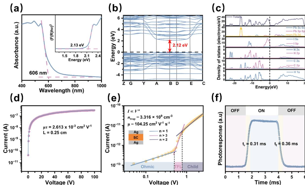
**Fig. 2** (a) Absorption spectra of MPI. The inset shows the diffuse-reflectance spectrum. The calculated electronic band structure (b) and DOS (c) of MPI. (d) The carrier mobility–lifetime ( $\mu\tau$ ) product of MPI. (e) Logarithmic  $I$ - $V$  curves were measured by using the SCLC method. (f) The rise and fall response times of an optical switch.
