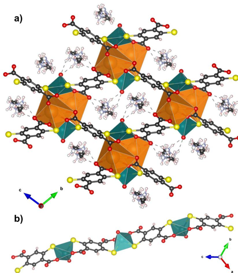
**Fig. 1** Crystalline structure of (DMA)KVO(DSBDC): (a) view along the *a* axis and (b) representation of the VO(DSBDC) 1-D chain. Vanadium, potassium, sulfur, oxygen, nitrogen, carbon and hydrogen are represented in dark green, orange, yellow, red, pale blue, black and white, respectively.
