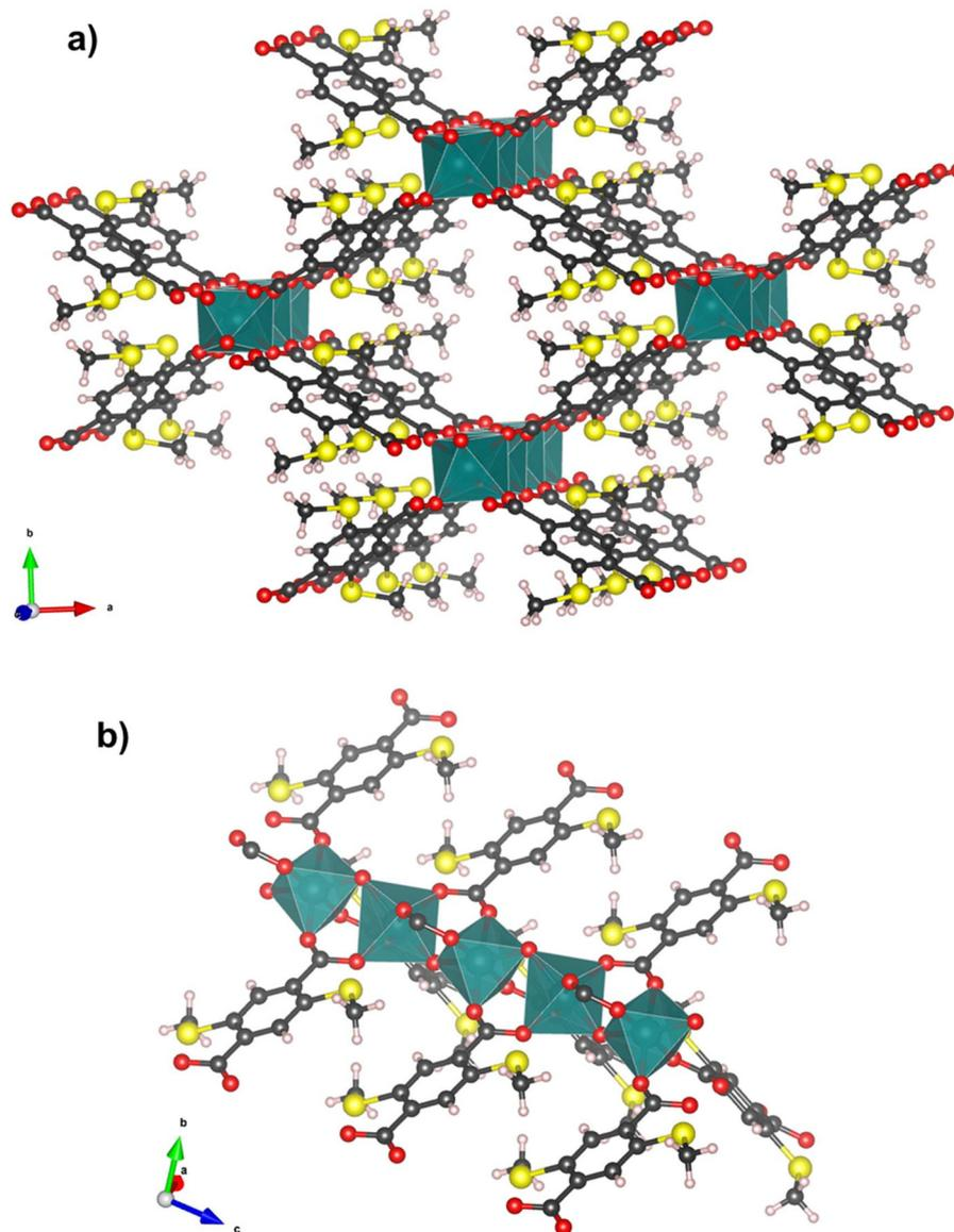
**Fig. 2** Structure of MIL-47(V)-( $SCH_3$ )<sub>2</sub> (a) and representation of the  $VO_6$  chains (b). Vanadium, sulfur, oxygen, carbon and hydrogen are represented in dark green, yellow, red, black and white, respectively. Entrapped DMF molecules are omitted for the sake of clarity.
