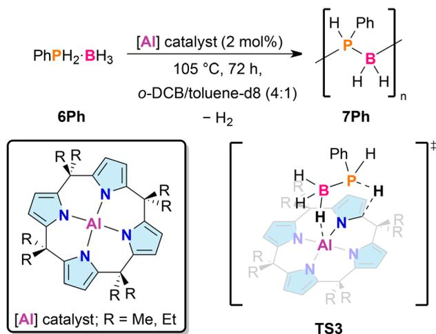
**Fig. 4** Dehydrocoupling of  $\text{PhPH}_2\text{-BH}_3$  using calix[4]pyrrolato aluminate as a catalyst. The proposed intermediate where P–H bond is acidified via a B–H–Al interaction (TS3) is also shown.
