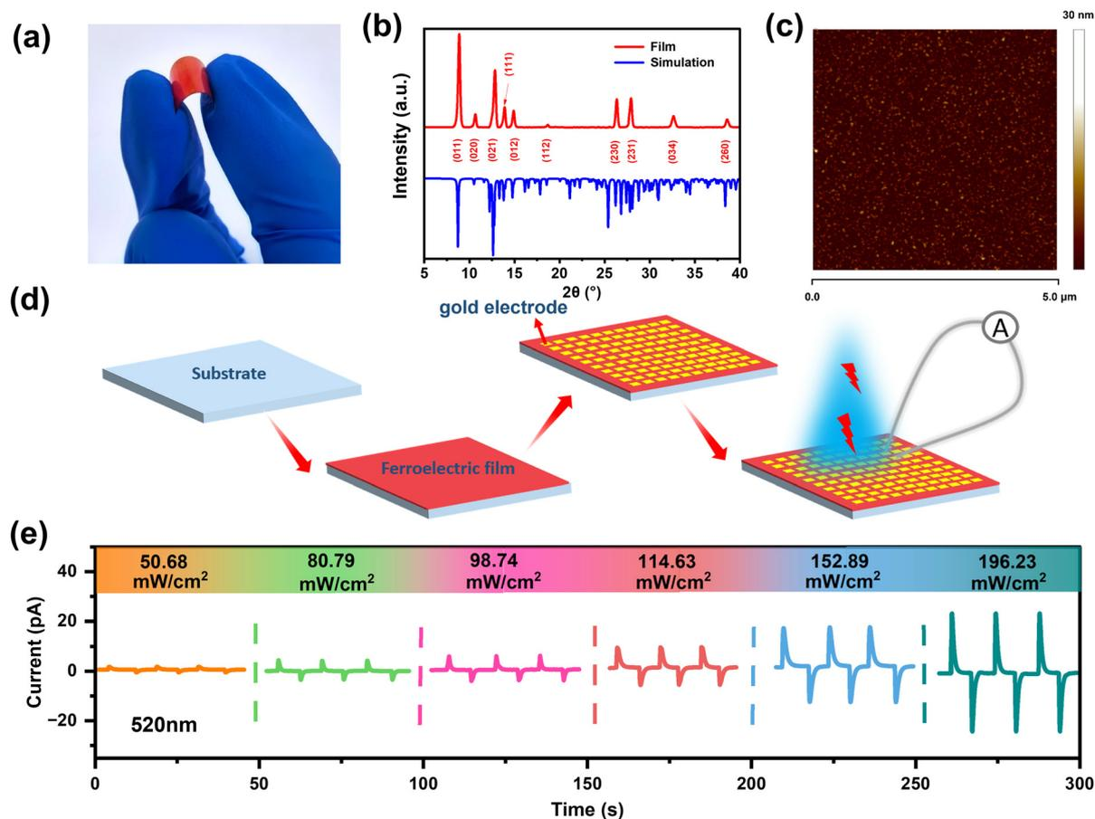
**Fig. 5** (a) Image of the flexible ferroelectric film of **1**. (b) XRD patterns of the ferroelectric film based on the substrate platform and theoretical data. (c) AFM image of the thin film of **1**. (d) Schematic diagram of the thin-film device fabrication process. (e)  $I-t$  curves measured under 520 nm laser irradiation with different densities at zero bias.
