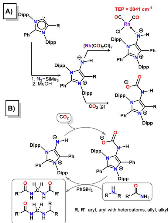
**Scheme 10** (A) Synthesis of aNHIs as reported by Mandal *et al.*, the reactivity thereof with CO<sub>2</sub>-gas and [Rh(CO)<sub>2</sub>Cl]<sub>2</sub> and the respective TEP determined. (B) Amide/amine-coupling with CO<sub>2</sub>, catalysed by an aNHI.<sup>71</sup>
