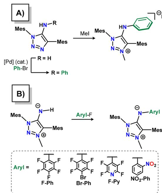
**Scheme 3** Possible methods for substitution of  $R^{exo}$  of MIIs. (A) Pre-functionalisation of 5-amino-1,2,3-triazoles by Buchwald–Hartwig amination. (B) C–F activation with electronpoor arylfluorides.<sup>71</sup>
