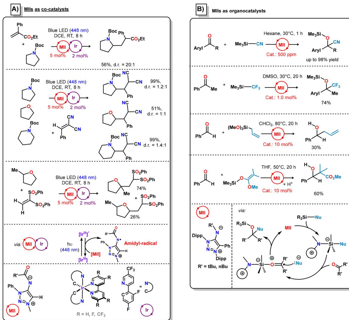
**Scheme 9** Application of MIIs. (A) As Co-catalyst in light-driven HAT with Ir<sup>III</sup>-complexes. (B) Addition of silyl-based nucleophiles on aromatic carbonyls under MII-catalysis.
