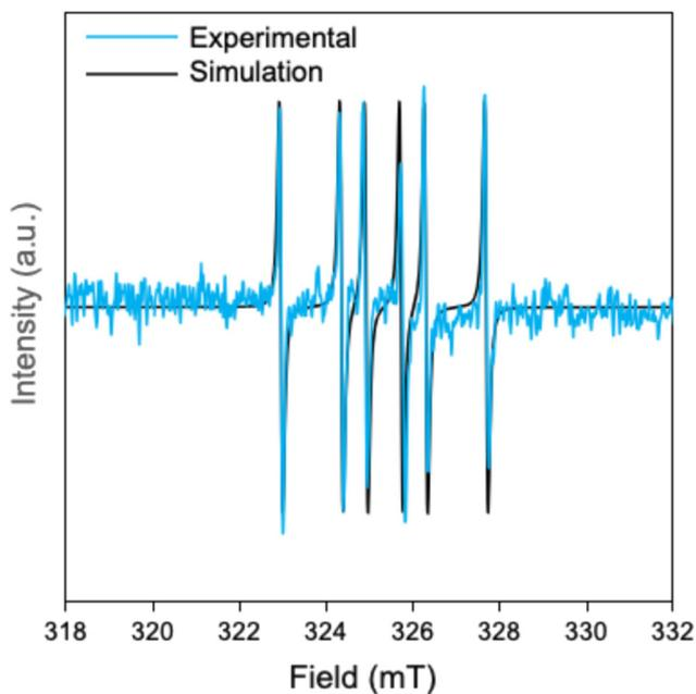
**Fig. 3** EPR spectrum of Grignard-metathesized Br-3MEEMT-Br quenched with DMPO in THF. Experimental (blue) and simulated (black) EPR spectra. Simulation parameters:  $A_N = 1.39$  mT,  $A_H = 1.96$  mT,  $g = 2.007$ . Microwave frequency: 9137.6 MHz; recorded at RT.
