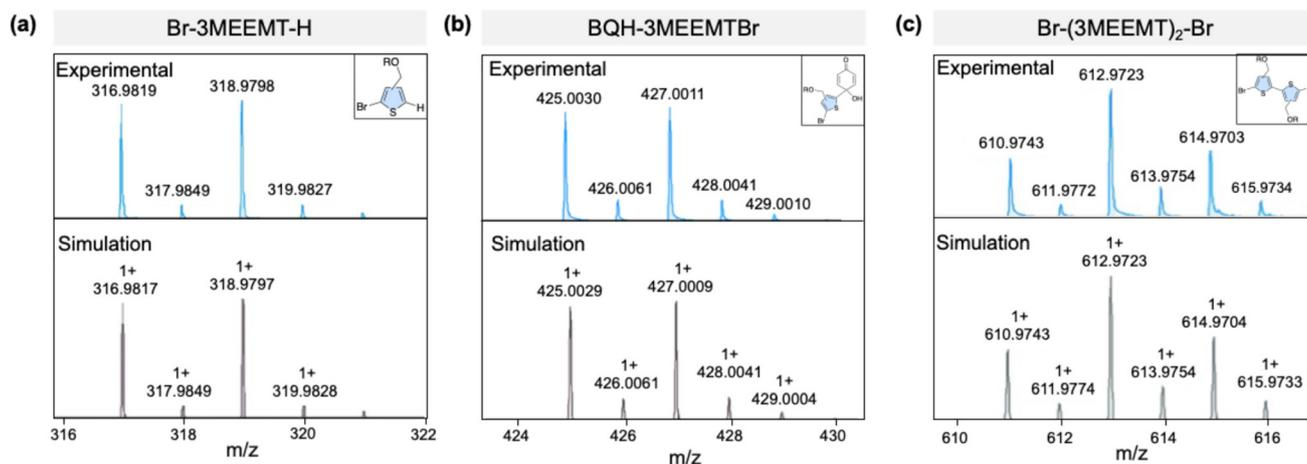
Fig. 4 (a) LC-MS spectra of the sodium salt of crude product of the Grignard-metathesized Br-3MEEMT-Br reaction with BQ in THF. (a) Br-3MEEMT-H, (b) BQH-3MEEMTBr, and (c) Br-(3MEEMT)<sub>2</sub>-Br.
