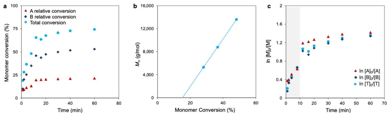
Fig. 6 (a) Monomer conversion vs. time, (b)  $M_n$  vs. monomer conversion, and (c)  $\ln([M]_0/[M])$  vs. time for polymerization conducted with  $\text{MgCl}_2$  (1 eq.) after the Grignard metathesis process.
