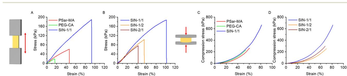
**Fig. 4** (A) Stress–strain plot of PSar-MA, PEG-CA, and SIN; (B) stress–strain plot of SIN-1/1, SIN-1/2 and SIN-2/1; (C) compressive stress of PSar-MA, PEG-CA, SIN; (D) compressive stress of SIN-1/1, SIN-1/2, and SIN-2/1. Total polymers concentration 30 wt% in NMP, BAPO 4 wt%.
