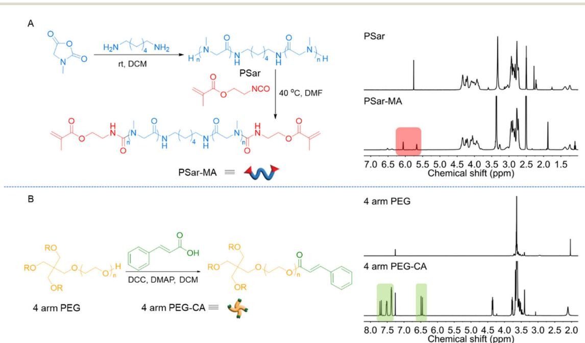
**Fig. 1** Synthetic procedure for the synthesis of (A) PSar-MA and (B) 4 arm PEG-CA and their <sup>1</sup>H NMR spectra. Red and green boxes in the <sup>1</sup>H NMR spectra highlight reactive methacrylate (MA) and cinnamic acid (CA) end-groups. Full peak assignment available in Fig. S2 and S3.
