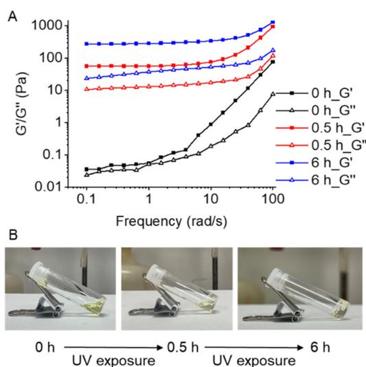
**Fig. 2** (A) Frequency sweep showing the viscoelastic behavior of the SIN-1/1 hydrogel over a range of angular frequencies at constant strain, with curves measured at different UV (405 nm) exposure timepoints. Storage modulus ( $G'$ , filled symbols) and loss modulus ( $G''$ , open symbols) (PSar-MA 15 wt%, PEG-CA 15 wt%, BAPO 4 wt%, NMP 70 wt%). (B) Gelation process of the PEG-CA hydrogel precursor solution over time (PEG-CA 15 wt%, BAPO 4 wt%, NMP 85 wt%).
