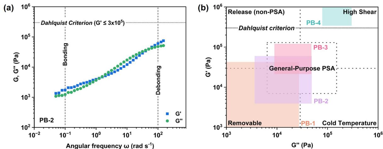
Fig. 2 (a) Frequency sweep of PB-2 (25 °C). (b) PSA performance windows of pentablock polyesters constructed from the bonding ( $\omega = 0.1$  rad s<sup>-1</sup>) and debonding frequencies ( $\omega = 100$  rad s<sup>-1</sup>).
