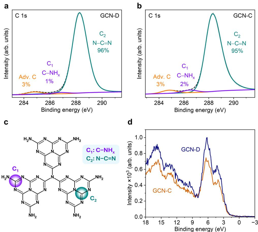
**Fig. 2** Deconvoluted high-resolution C 1s core-level XPS spectra of (a) GCN-D and (b) GCN-C. (c) The structure of GCN highlighting C<sub>1</sub> and C<sub>2</sub> sites and (d) VB-XPS spectra of GCN-D and GCN-C.
