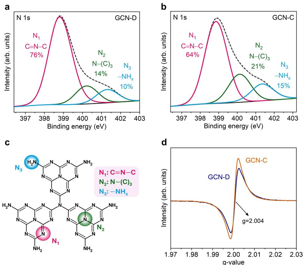
**Fig. 3** Deconvoluted high-resolution N 1s core-level XPS spectra of (a) GCN-D and (b) GCN-C. (c) The structure of GCN highlighting  $N_1$ ,  $N_2$  and  $N_3$  sites and (d) EPR spectra of GCN-D and GCN-C.
