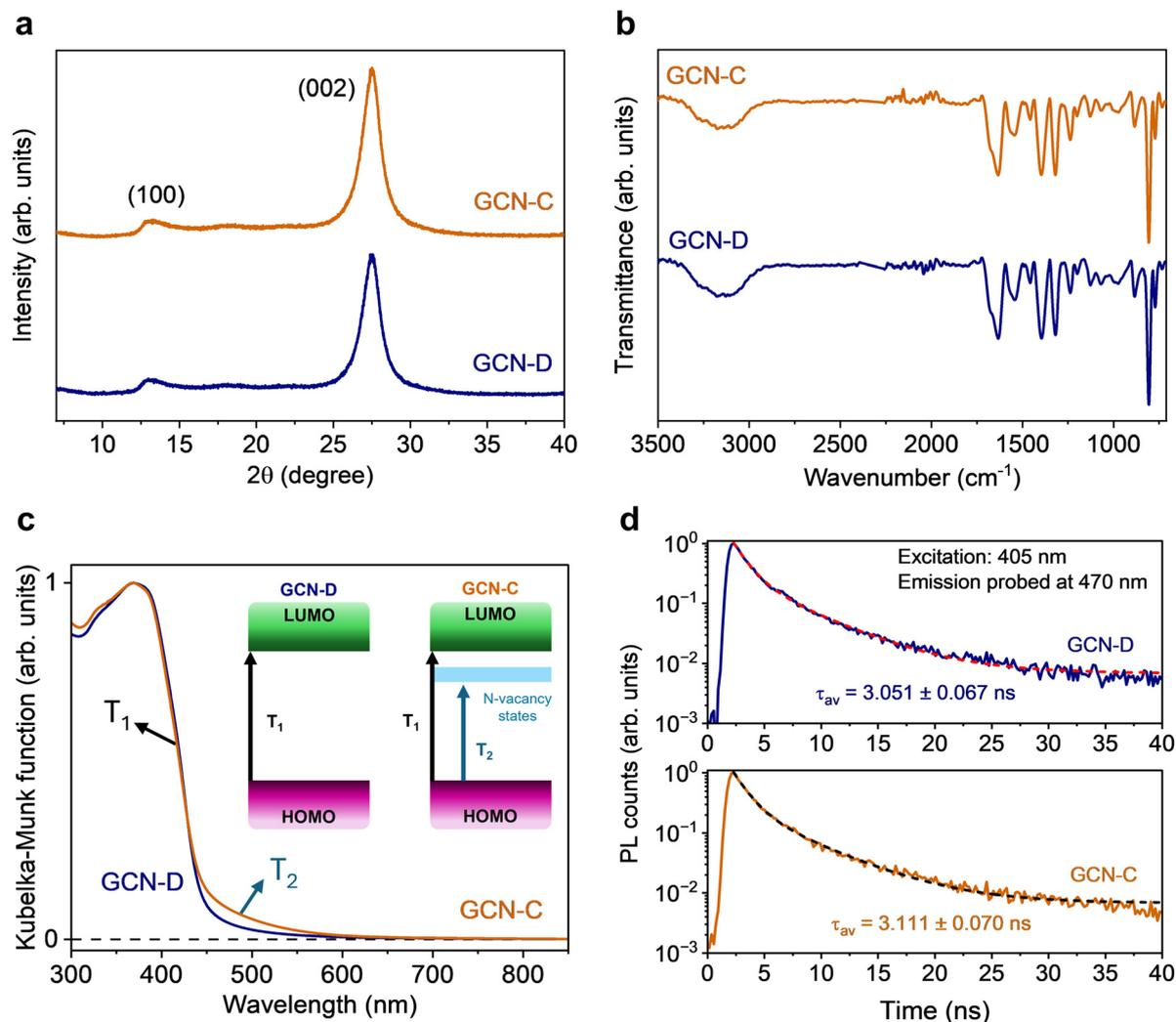
**Fig. 1** (a) XRD patterns, (b) FTIR spectra, (c) optical absorption spectra measured in diffuse reflectance mode (inset: electronic transitions), and (d) time-resolved PL (tr-PL) transients of GCN-D and GCN-C. The dotted lines in the transient plots are a result of biexponential function fitting.
