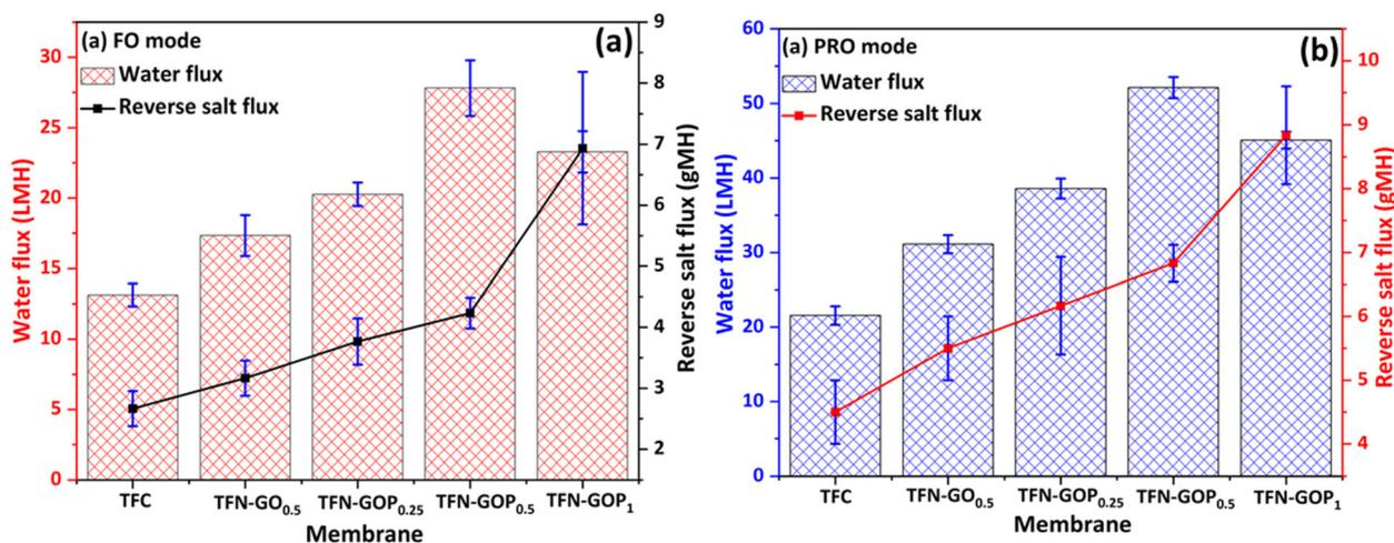
Fig. 11 Water flux ( $J_w$ ) and reverse salt flux ( $J_s$ ) of TFC and GO/GO-g-PDMA-modified TFN-FO membranes in (a) FO mode and (b) PRO mode. Tests are performed using a 1 M NaCl draw solution and DI water as the feed.
