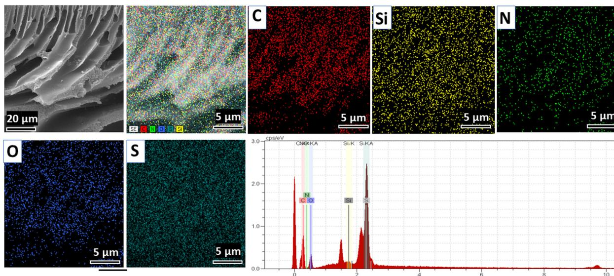
Fig. 10 EDS elemental mapping images of the TFN-GOP<sub>0.5</sub> membrane.
