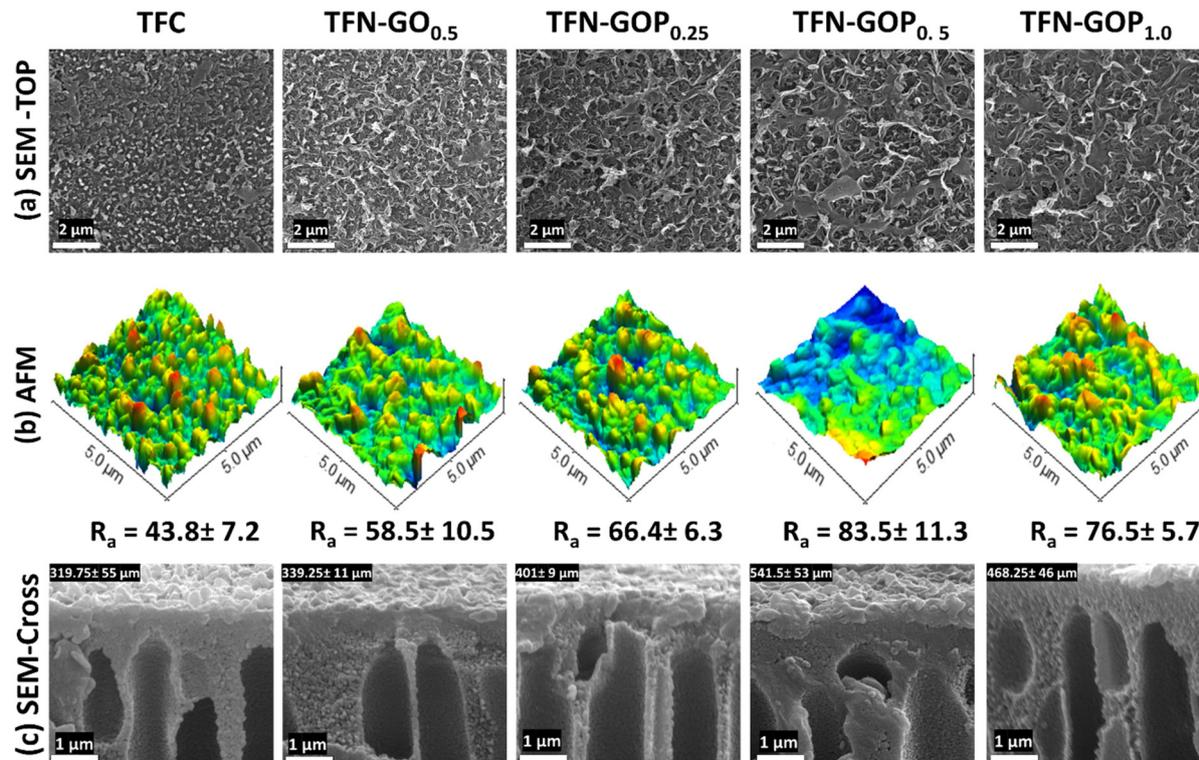
**Fig. 9** (a) Top surface SEM images showing the morphological differences in the PA layers of TFC and TFN-FO membranes; (b) three-dimensional AFM images depicting changes in surface roughness with increasing GO-g-PDMA content; and (c) cross-sectional SEM images illustrating the overall membrane structure and thickness of the PA layers formed on different substrates.
