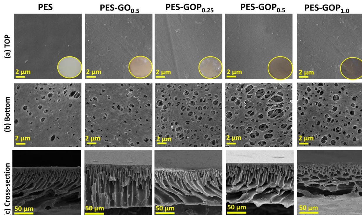
**Fig. 6** (a) SEM images of the top surface morphologies and corresponding digital photographs of the substrates; (b) SEM images of the bottom surface morphologies; and (c) cross-sectional SEM images of the substrates.
