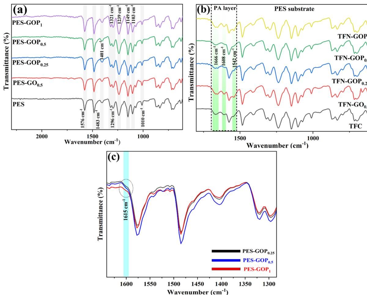
**Fig. 5** ATR-FTIR spectra of (a) the prepared PES-based substrates containing GO and GO-*g*-PDMA nanofillers, (b) the fabricated TFC and TFN-FO membranes, and (c) magnification of the support layer ATR-FTIR spectra.
