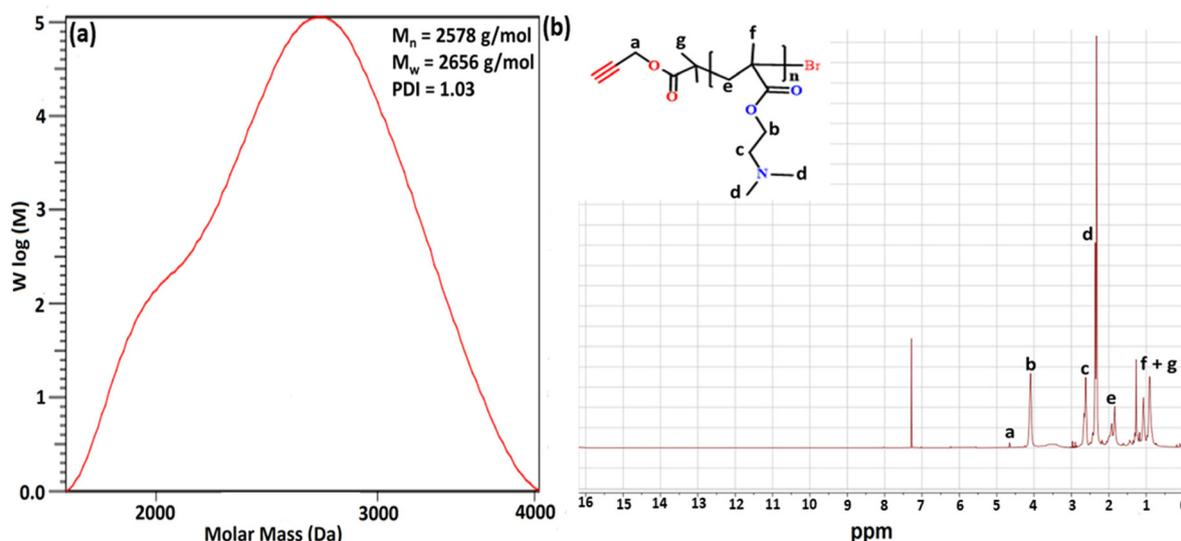
Fig. 2 (a) GPC chromatogram and (b)  $^1\text{H}$  NMR spectrum of the alkyne-terminated PDMA polymer.
