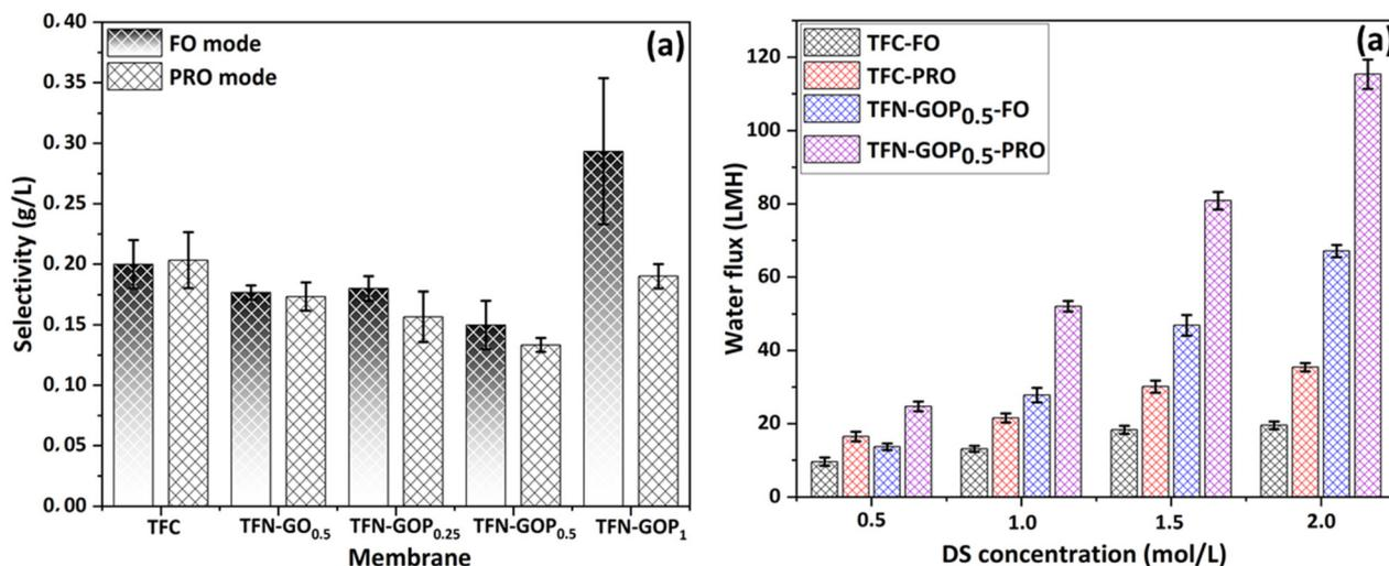
Fig. 12 (a) Selectivity ( $J_s/J_w$ ) of the TFC and TFN-FO membranes in FO and PRO modes. (b) Effect of DS concentration on the water flux of TFC and TFN-GOP<sub>0.5</sub> membranes.
