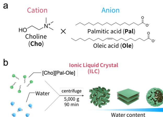
Fig. 1 Design of the ionic liquid crystal (ILC) system. (a) Structural formula of ionic liquids (ILs). (b) ILC preparation scheme.
