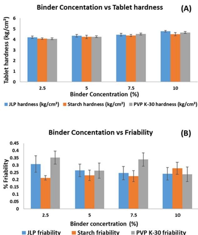
Fig. 7 Mechanical strength of tablets prepared using JLP as a binding agent: (A) binder concentration vs. tablet hardness and (B) binder concentration vs. friability.
