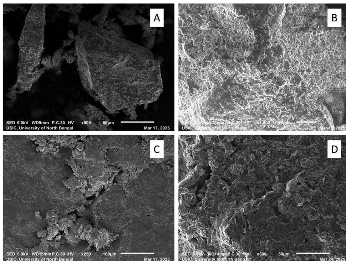
**Fig. 6** SEM images of (A) dried JLP powder particles at 500x magnification; (B) JLP powder particles at higher magnification (1500x); (C) compressed tablet surface before dissolution; and (D) porous surface during tablet dissolution.
