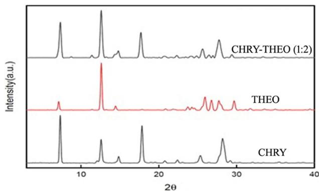
**Fig. 5** PXRD patterns of CHRY, THEO and the CHRY-THEO (1:2) eutectic mixture.
