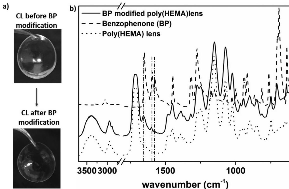
**Fig. 4** (a) Contact lens appearance before and after modification with BP; (b) ATR-FTIR spectra of lens before and after modification with BP (new peaks on BP-modified lens indicated by vertical dotted lines).
