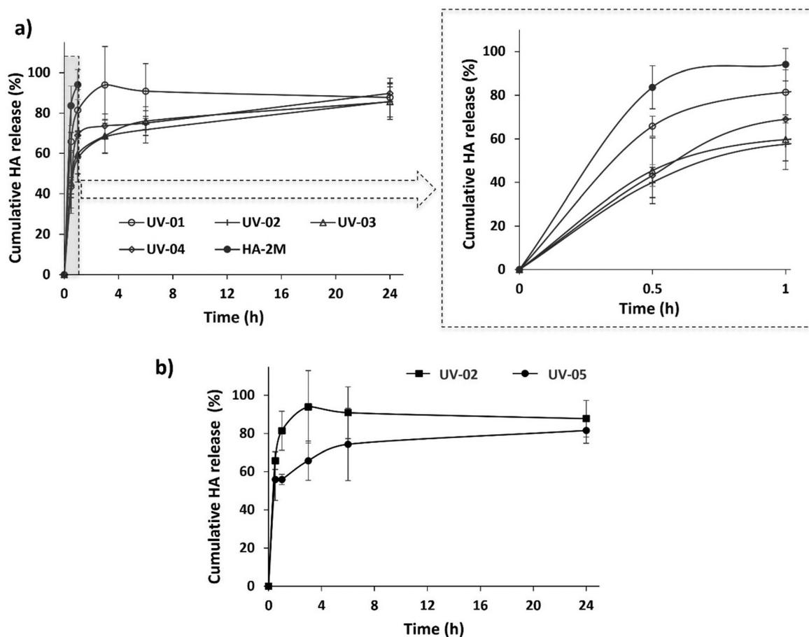
**Fig. 5** (a) Cumulative HA release (%) of the lenses with the printed semi-IPN polymer ring using different monomers (HEMA and DEAEMA or a mixture of both) and crosslinker (PEGDA<sub>700</sub>) ratios, with the enlarged display of the release profile of the first hour (insert on the right); (b) HA release of lens UV-05 with a lower MW crosslinker, PEGDA<sub>575</sub>, in comparison to UV-02 (data are presented as mean  $\pm$  SD;  $n = 3$ ).
