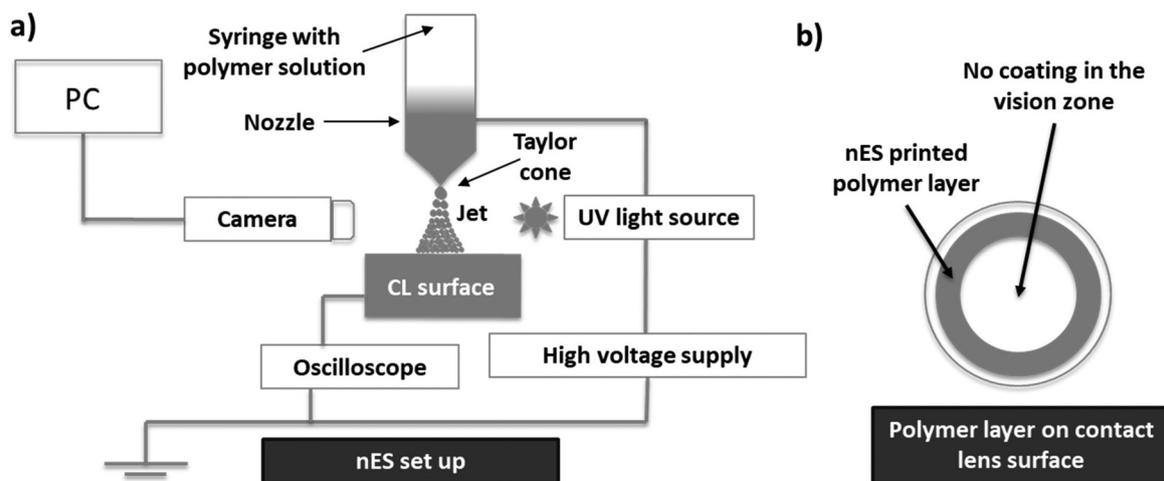
**Fig. 3** nES setup was used for depositions on contact lenses. Schematic illustration (a) of the nES setup; (b) polymer layer printed at the periphery of contact lens via nES.
