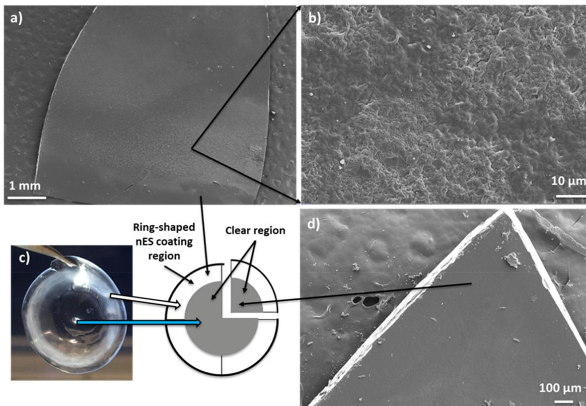
**Fig. 7** (a) A representative cryo-SEM image of the bilayer (semi-IPN as a base coat and zein as a top coat) deposited layer at the periphery on BP-modified lens; (b) higher resolution of the surface of the bilayer-coated lens; (c) visual appearance of a bilayer-coated lens and schematic diagram to show the cryo-SEM sampling location; (d) cryo-SEM image of the center of contact lens (not coated) having a smooth surface with no polymer coating.
