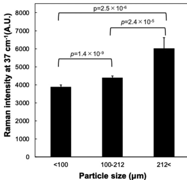
Fig. 7 Effect of particle size on Raman peak intensity at  $37\text{ cm}^{-1}$  in tablets composed entirely of carbamazepine Form III ( $N = 3$ , error bars represent the standard deviation). Larger particles exhibited stronger but more variable signals, while smaller particles produced more consistent results.
