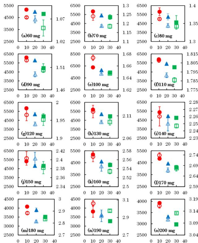
Fig. 4 Relationship between signal intensity and tablet thickness measured at an exposure time of 1 s, categorized by sample mass ( $N = 3$ , error bars represent the standard deviation of three measurements). The left vertical axis represents Raman spectral intensity, the right vertical axis represents tablet thickness (mm), and the horizontal axis represents tablet pressure (MPa). ● : 10 MPa, ▲ : 20 MPa, and ■ : 30 MPa (hollow symbols represent tablet thickness).
