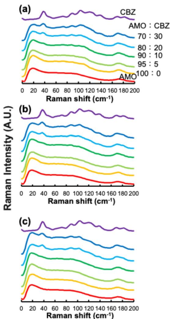
Fig. 6 Correlation between carbamazepine (CBZ) Form III concentration and Raman spectral intensity in CBZ\_amo tablets at different particle size ranges: (a)  $\leq 100$   $\mu\text{m}$ , (b) 100–212  $\mu\text{m}$ , and (c)  $>212$   $\mu\text{m}$ . Increasing crystalline content led to distinct spectral peaks.
