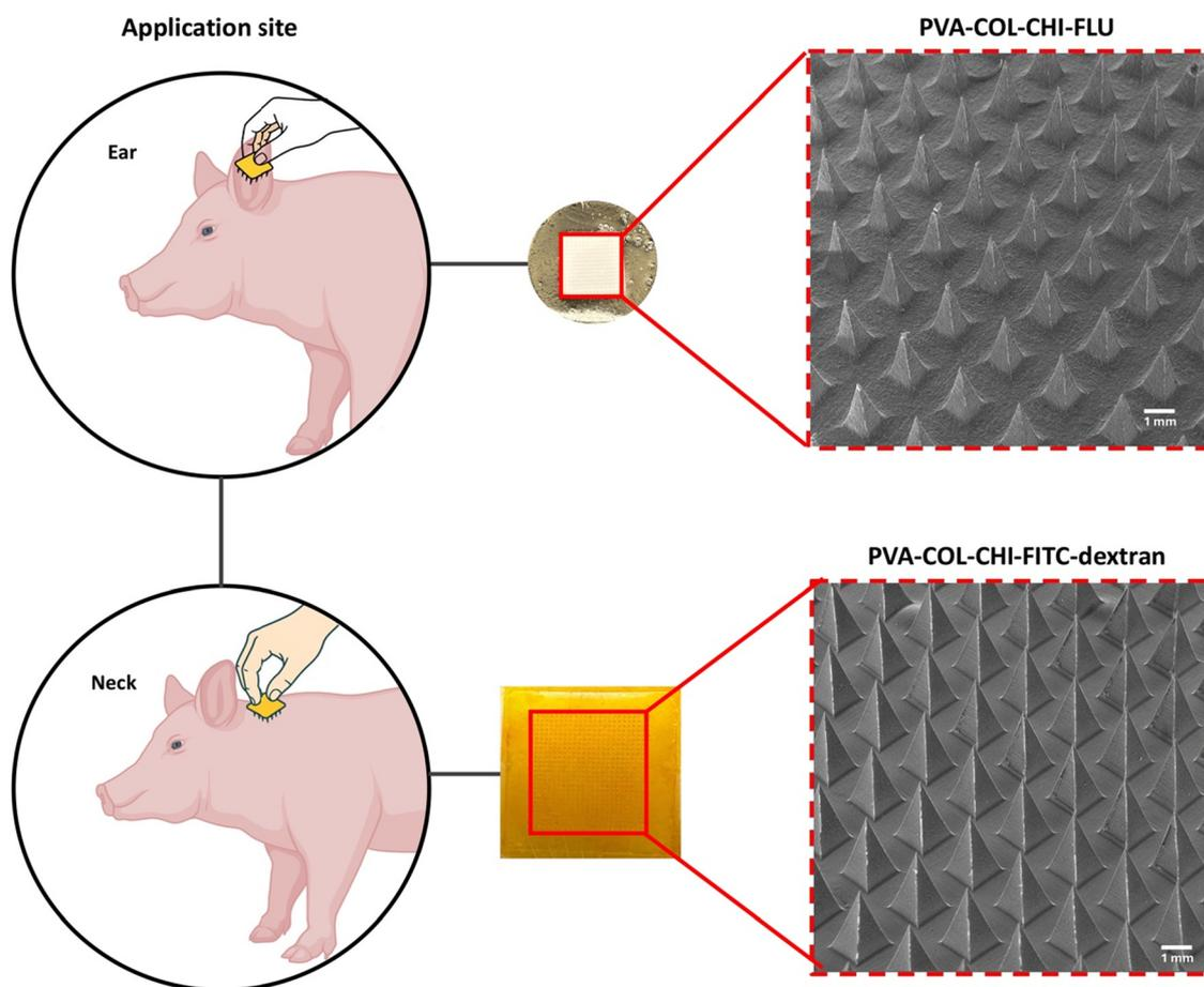
**Fig. 2** Application sites and morphological analysis of microneedle patches. Macroscopic (center) and SEM (right) images of PVA-COL-CHI patches loaded with FLU or FITC-dextran highlight the consistent microneedle geometry.
