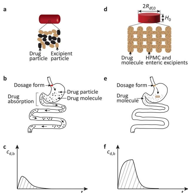
**Fig. 1** Schematics of dosage form microstructure, passage through the gastrointestinal tract, and drug concentration in blood after single dosing: (a)–(c) particulate dosage form, and (d)–(f) solid-solution fibrous dosage form.  $c_{d,b}$ : drug concentration in blood;  $t$ : time. Bioavailability is the area under the curve.
