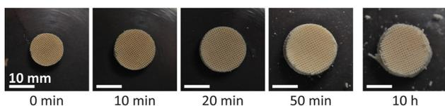
**Fig. 4** Top-view images of a fibrous dosage form at various times after immersing in a dissolution fluid.
