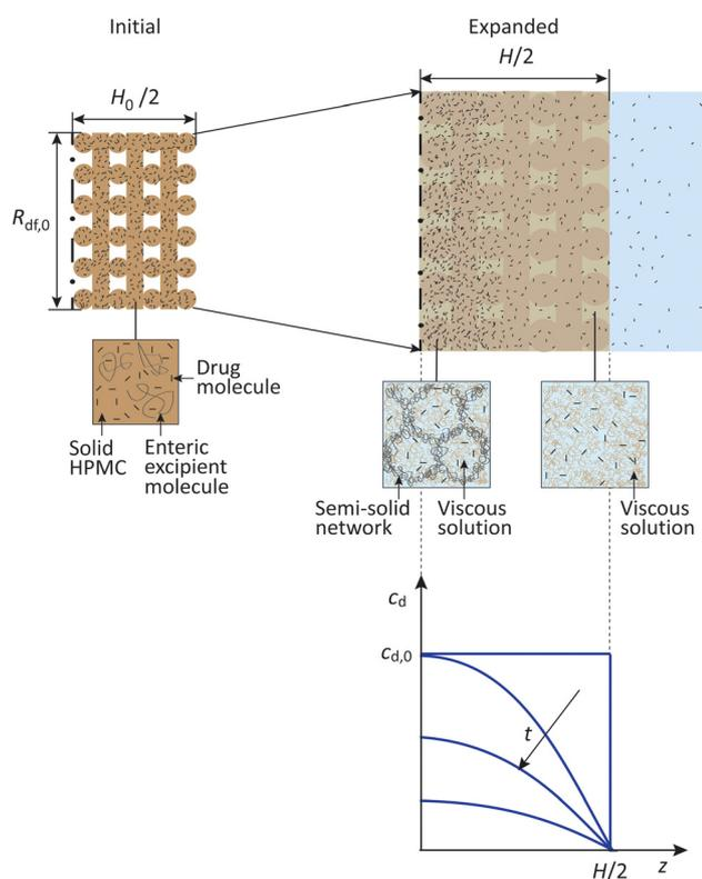
**Fig. 7** Schematic microstructures of the initial and expanded dosage forms, and drug concentration profile in the expanded dosage form at various times. In the experiments, the radius and thickness of the initial dosage forms were:  $R_{df,0} = 7$  mm and  $H_0 = 6.5$  mm. For illustrative purpose the drug molecules are shown in both the schematic microstructures of the fibrous dosage forms, and the enlargements of the fibers and the inter-fiber space.
