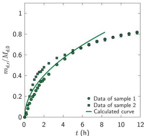
**Fig. 6** Measured and calculated fraction of drug released,  $m_{d,r}/M_{d,0}$ , versus time,  $t$ , after immersing fibrous dosage forms in the dissolution fluid. The calculated curve is from eqn (8) using the parameter values of Appendix B. The data represent two samples.
