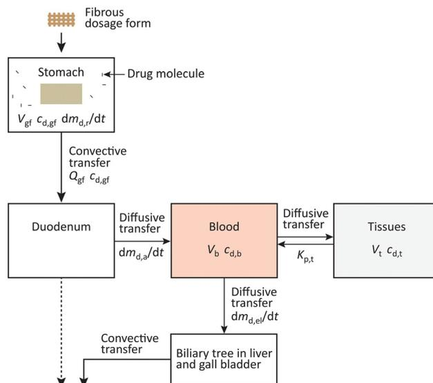
**Fig. 11** Block diagram of drug release, absorption by the blood, interdiffusion with tissues, and elimination. The absorption rate,  $dm_a/dt = Q_{gf}c_{d,gf}$ , and the elimination rate,  $dm_{el}/dt = (V_b + K_{p,t}V_t)c_{d,b}/\tau_{el}$ .<sup>27</sup>
