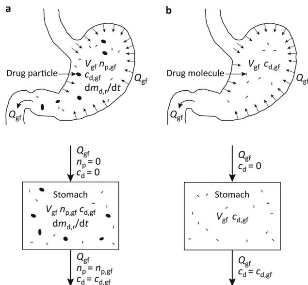
**Fig. 15** Schematic of mass flow rates into and out of the stomach after administering particulate dosage forms: (a)  $t < t_{r,p}$  and (b)  $t \gg t_{r,p}$ . Here  $t_{r,p}$  is the residence time of drug particles in the stomach. The schematic is reproduced from ref. 27.
