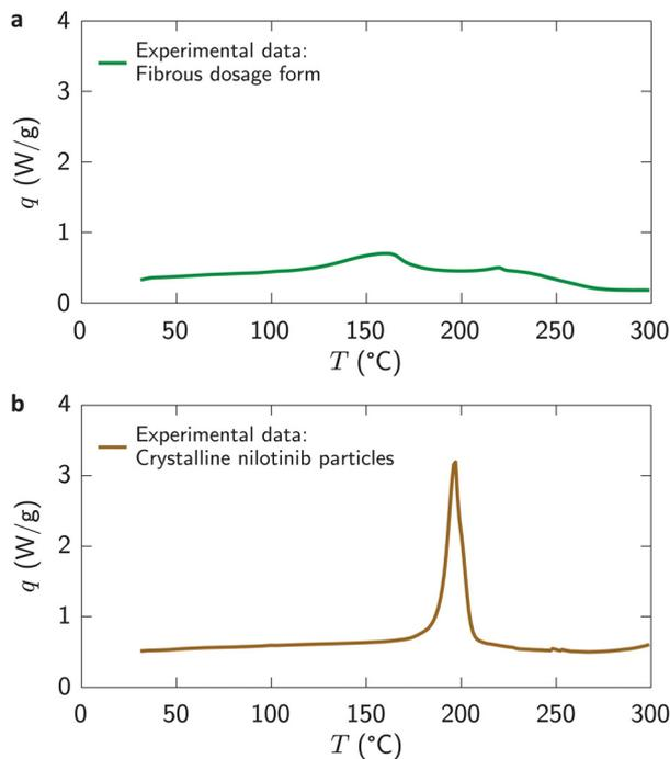
**Fig. 3** Specific heat flow,  $q$ , versus temperature,  $T$ , into: (a) drug-laden fibers of a solid-solution fibrous dosage form and (b) the solid particles of nilotinib hydrochloride monohydrate used for preparing the fibrous dosage forms.
