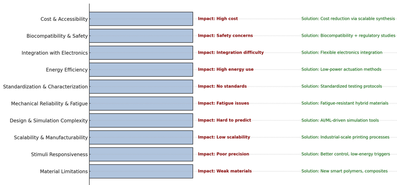
Fig. 12 Possible solutions to the problems that have so far plagued 4D printing.
