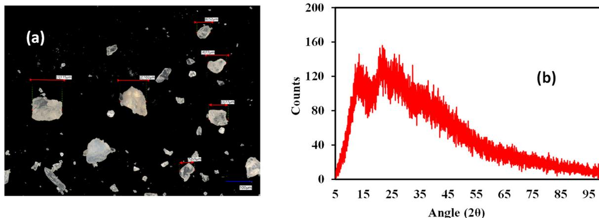
Fig. 2 Measurement of the grain width of the baobab polysaccharide with two-point measurement. (a) Original image of the grain sample  $\times 300$ . Scale bar is 100  $\mu\text{m}$ . (b) XRPD pattern of the extracted and milled baobab polysaccharide from a <250  $\mu\text{m}$  sieve.
