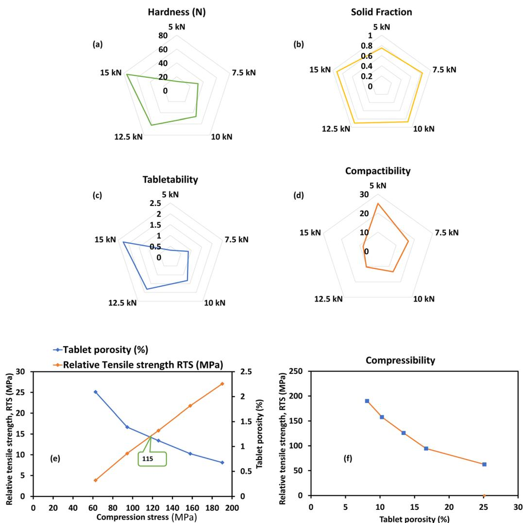
Fig. 4 Properties of compacted baobab polysaccharide (milled baobab polysaccharide from a <250  $\mu\text{m}$  sieve) under 5 kN–15 kN: (a) compact hardness, (b) solid fraction, (c) tableability, (d) compactibility, (e) compression stress relationship with tablet porosity and relative tensile strength and (f) tablet porosity relationship with tensile strength. All experiments were conducted in triplicate.
