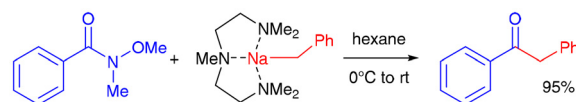
Scheme 1 Ketone synthesis from a Weinreb amides and a benzyl sodium reagent in a batch reaction.
