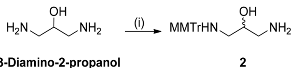
Scheme 1 Synthesis of tritylated diamino conjugator 2 . Reagents and conditions: (i) MMTr-Cl (1.0 eq.), DBU (3.0 eq.), MeCN, 22 °C, 1 h, 52%.
